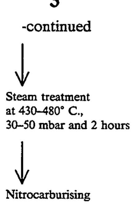
As a general proposition, the steam treatment according to the invention should be carried out at a temperature below 560° C., and preferably below 500° C., and 15 most preferably between 430° and 480° C., in order to prevent the formation of FeO and the subsequent decomposition upon cooling into Fe<sub>3</sub>O<sub>4</sub> and FeO, with the attendant disadvantages as previously discussed.
