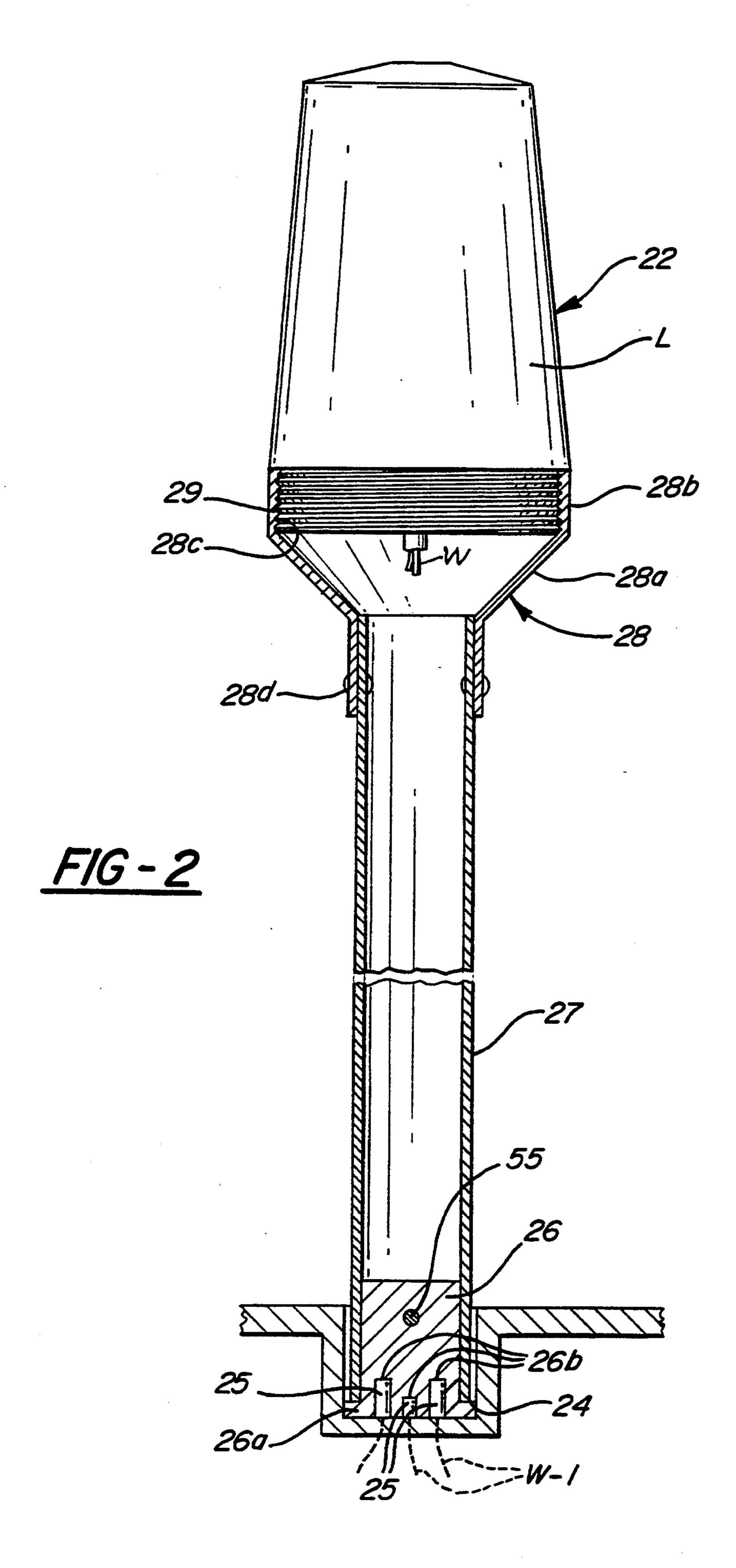
METHOD AND APPARATUS FOR WARNING OTHER BOATS IN THE PROXIMITY OF A WATER CRAFT FOR TOWING WATER SKIERS AND OTHER PERSONS TO BE TOWED THAT THE WATER SKIER IS DOWN OR THE PERSON IS INACTIVE IN THE WATER
