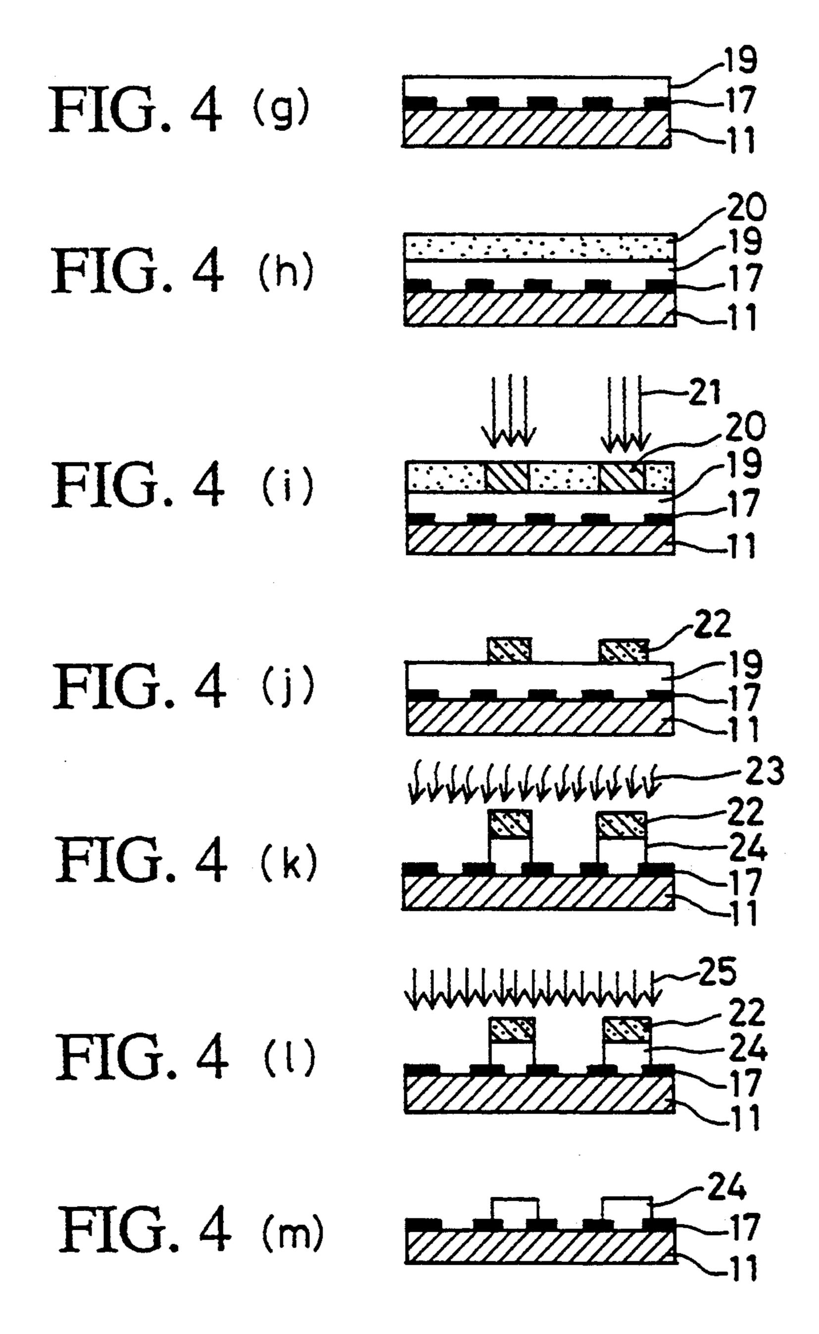
METHOD FOR FABRICATING PHOTOMASKS HAVING A PHASE SHIFT LAYER COMPRISING THE USE OF A POSITIVE TO NEGATIVE RESIST, SUBSTRATE IMAGING AND HEATING
