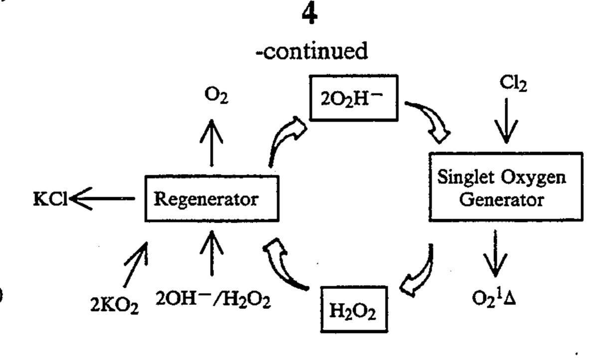
The primary alternative for the generation of BHP is the standard potassium hydroxide and hydrogen peroxide mixing reaction shown in eq. (1). This older generation method is significantly less expensive than these new proposed methods, but it would require additional chemical sources if the potassium superoxide regeneration method be used.
