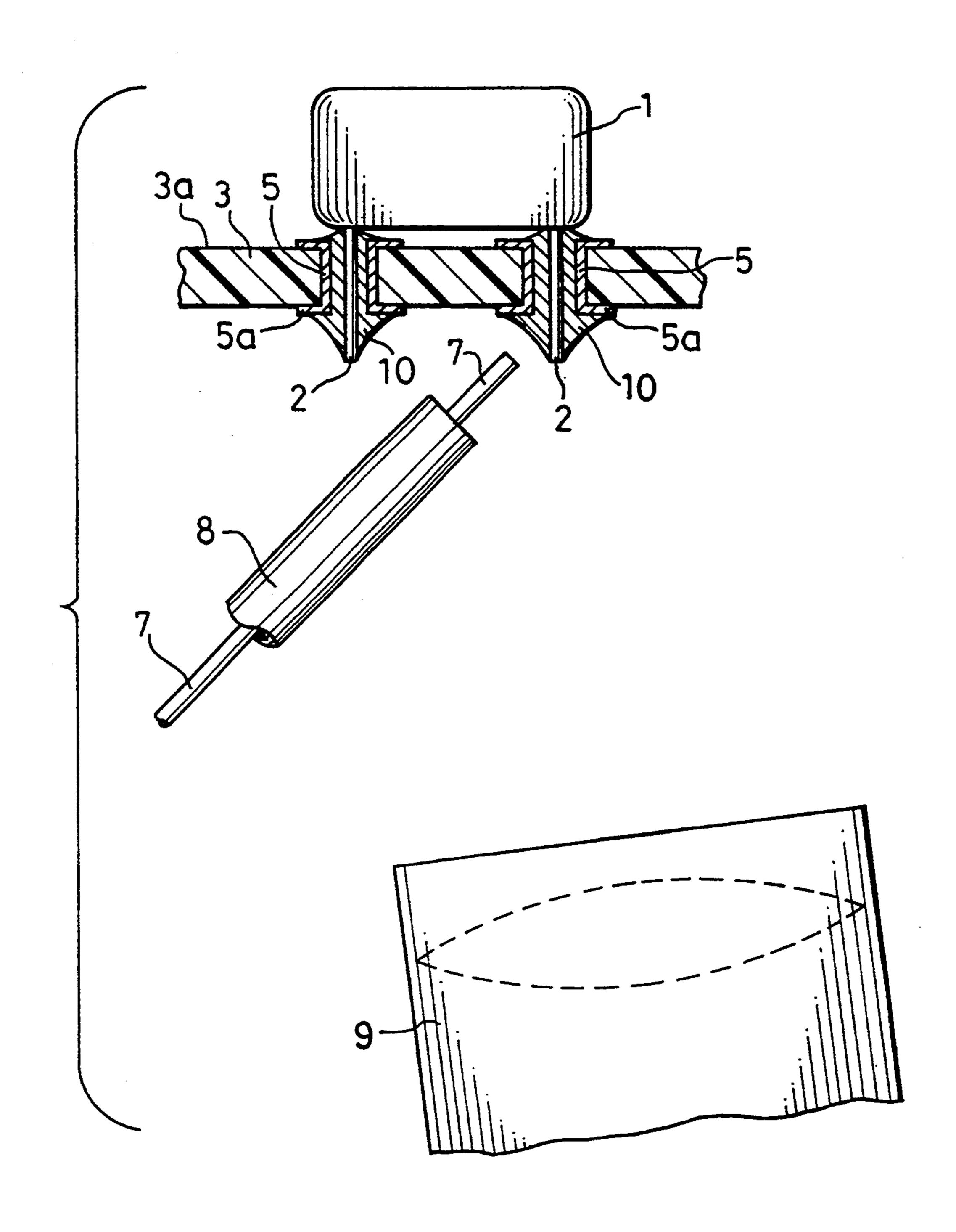
**UPWARD SOLDERING METHOD**
