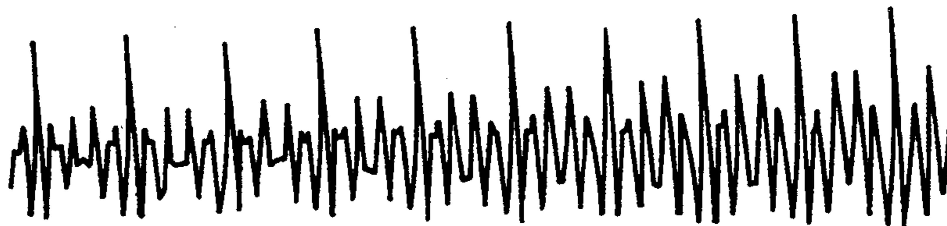
HIGH FREQUENCY WAVEFORM OF SYNTHESIZED SPEECH BY ZERO PHASE SETTING METHOD
