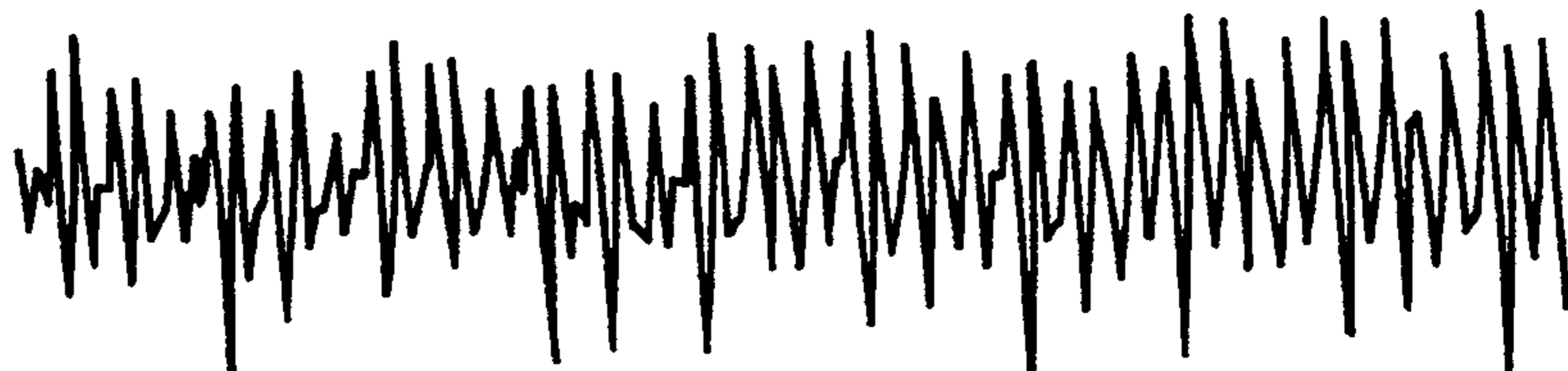
HIGH FREQUENCY WAVEFORM OF SYNTHESIZED SPEECH BY THE PRESENT INVENTION
