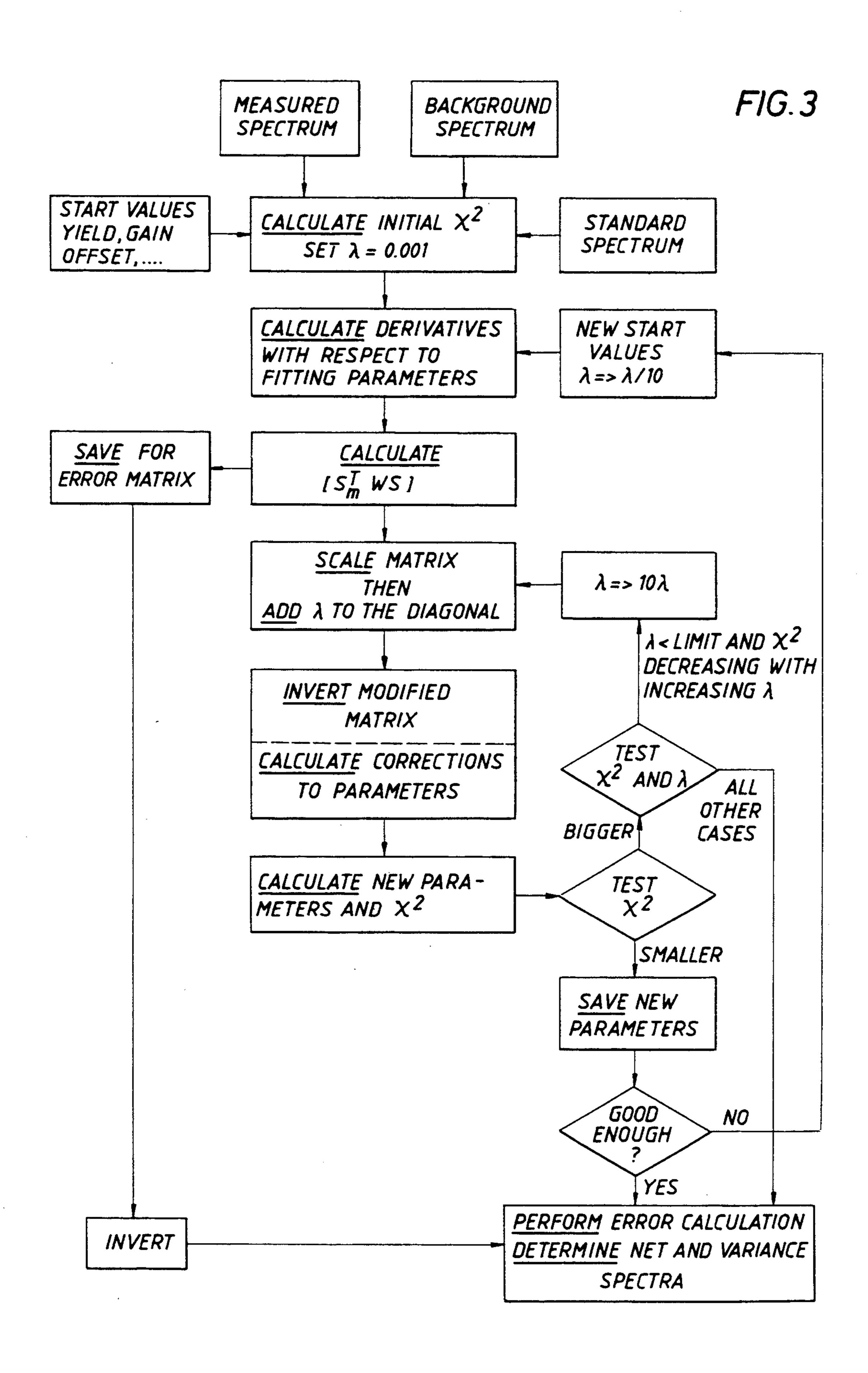
METHOD AND APPARATUS FOR USING NON-LINEAR SPECTRAL FITTING PROCEDURES ON GAMMA-RAY SPECTRAL DATA
