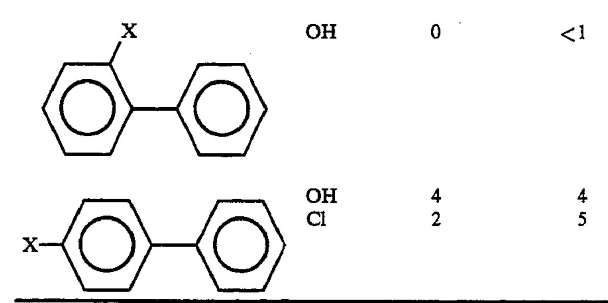
1. All reactions at 410° C., 4:1:0.1 weight ratio of donor to Ar—X to carbon catalyst. Ar—X represents an aryl compound substituted with a moiety designated as X.
