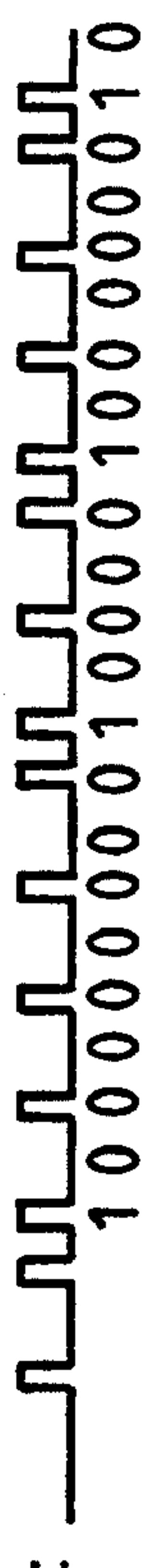
FIG. 21E LASER PULSE OF SEMICONDUCTOR LASER 51b (MODULATION SIGNAL)
