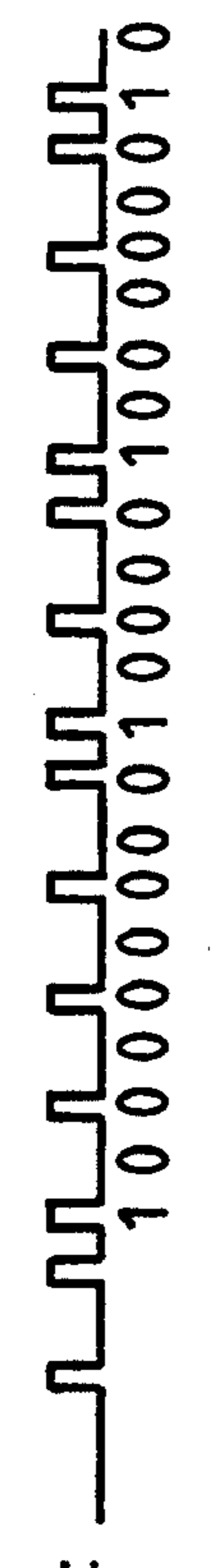
FIG. 21E LASER PULSE OF SEMICONDUCTOR LASER 51b (MODULATION SIGNAL)
