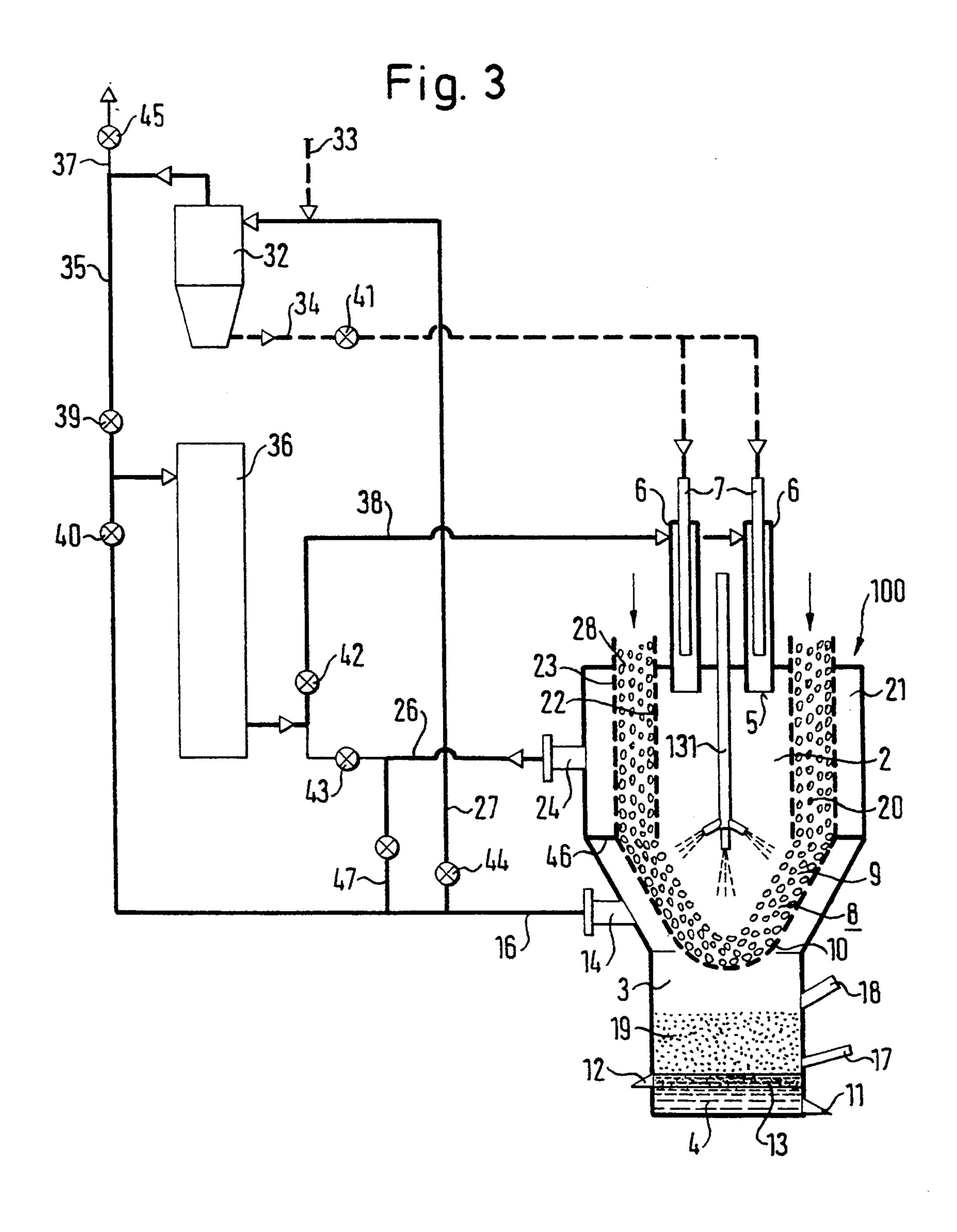
PROCESS FOR THE PRODUCTION OF LIQUID METAL FROM FINE-GRAIN METAL OXIDE PARTICLES AND REDUCING AND SMELTING FURNACE FOR CARRYING OUT THE PROCESS
