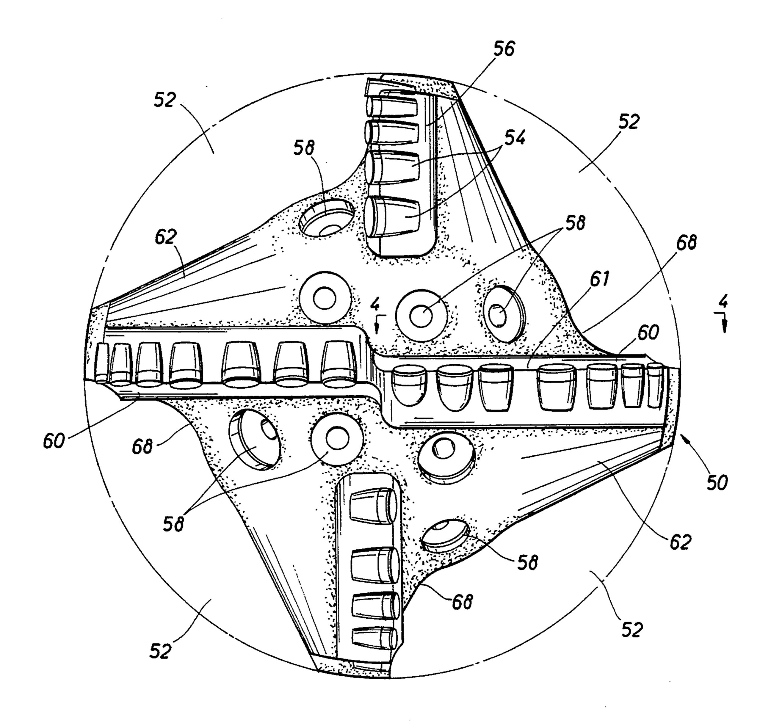
PDC DRAG BIT WITH IMPROVED HYDRAULICS
