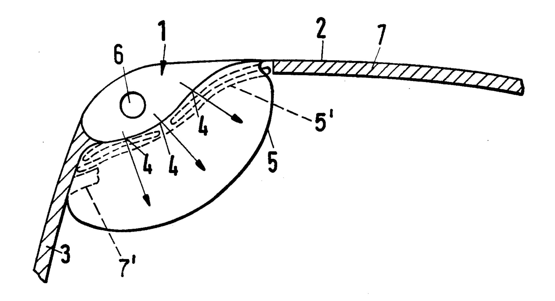
AIRBAG DEVICE MOUNTED IN A ROOF FRAME **REGION OF A VEHICLE**
