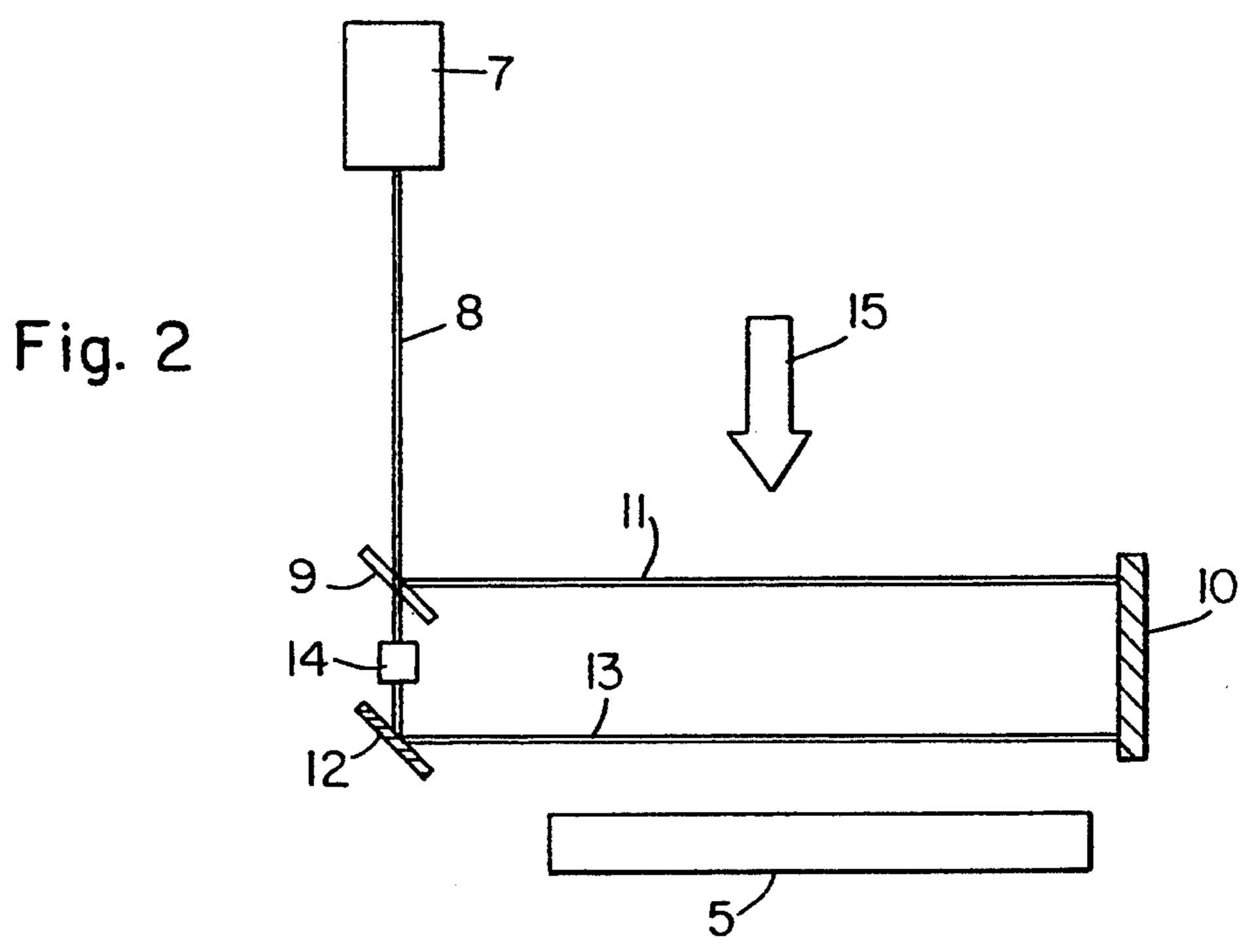
collimating and optically pumping the beam of atoms
