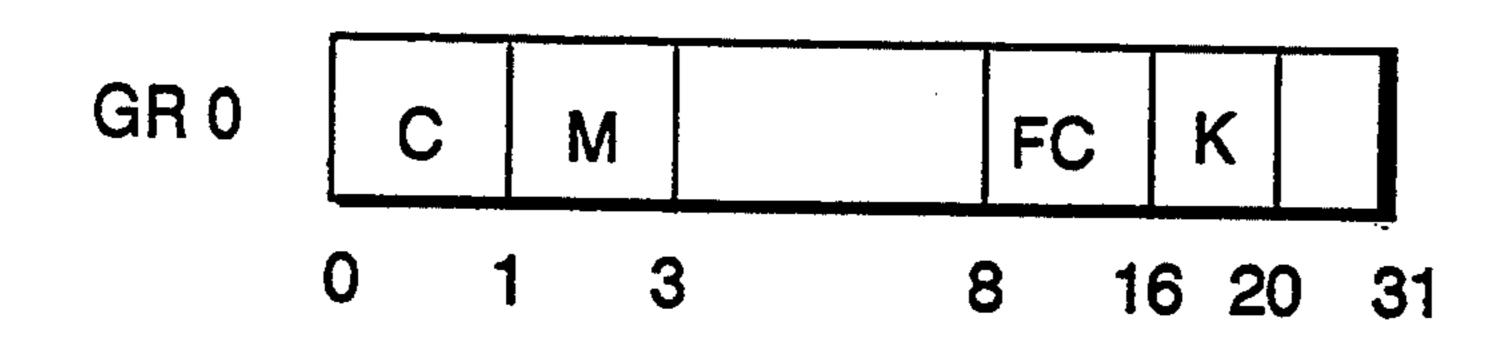
C = CONT. BIT 0M = 1-2 BITS MODE FC = 8-15K = 16-19 ACCESS KEY
