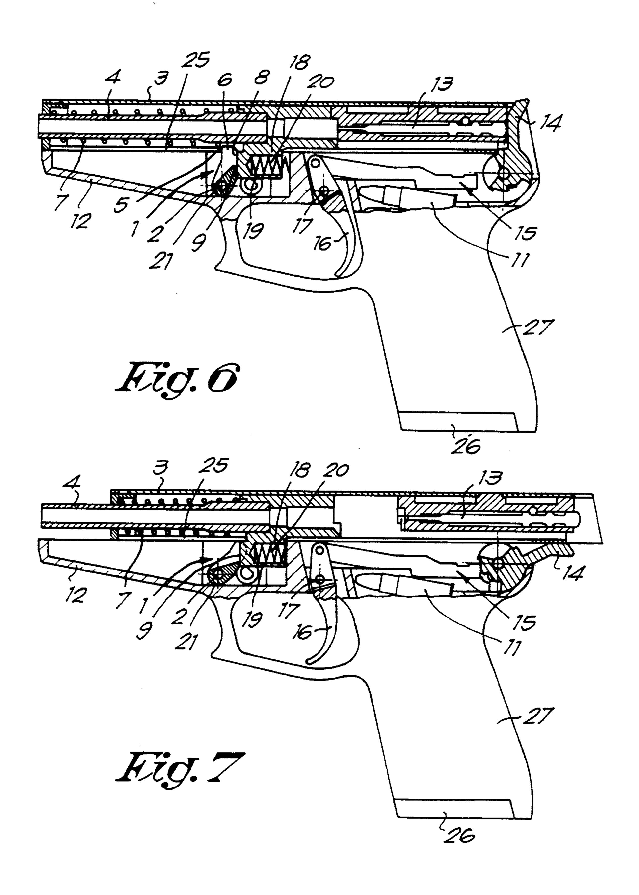
ELEMENTS FOR DECELERATING THE RECOIL OF THE MOVING PARTS OF A FIRE ARM
