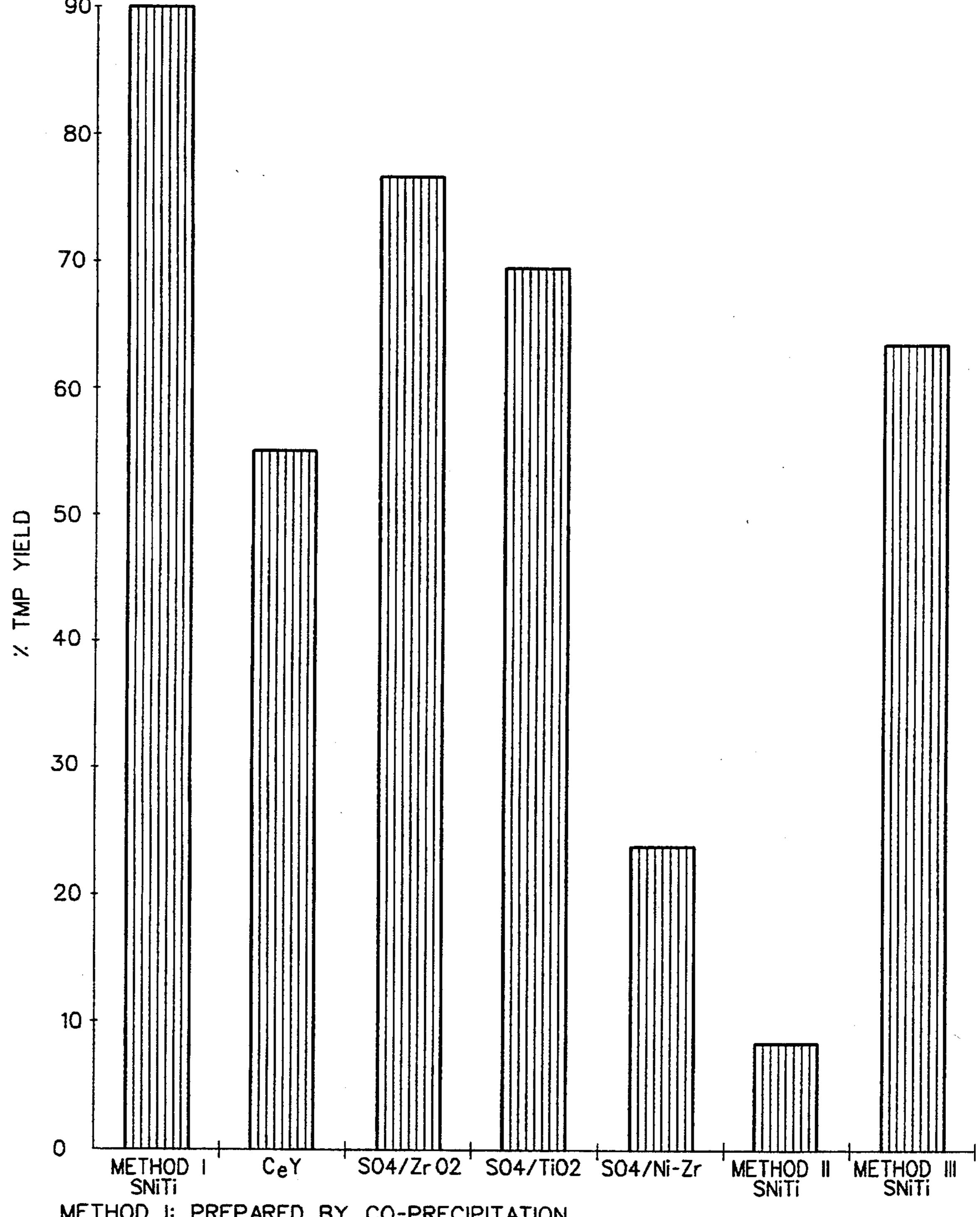
METHOD I: PREPARED BY CO-PRECIPITATION METHOD II: PREPARED BY IMPREGNATING TI(OH)4 WITH NI METHOD III: PREPARED BY IMPREGNATING TIO2 WITH NI
