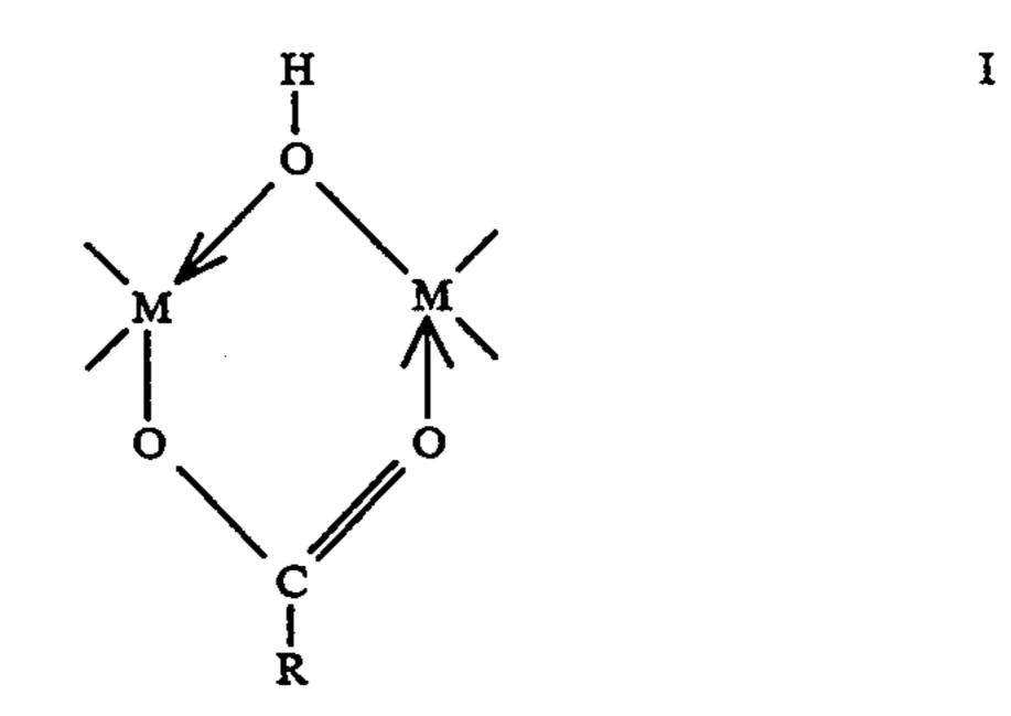
wherein M represents a chelate-forming metal atom and R represents an alkyl group. The fiber has excellent resistance to hot water and wet heat and does not stick, adhere or shrink even when dyed at high temperatures or treated by steam ironing, thus proving to be of markedly high commercial value.
