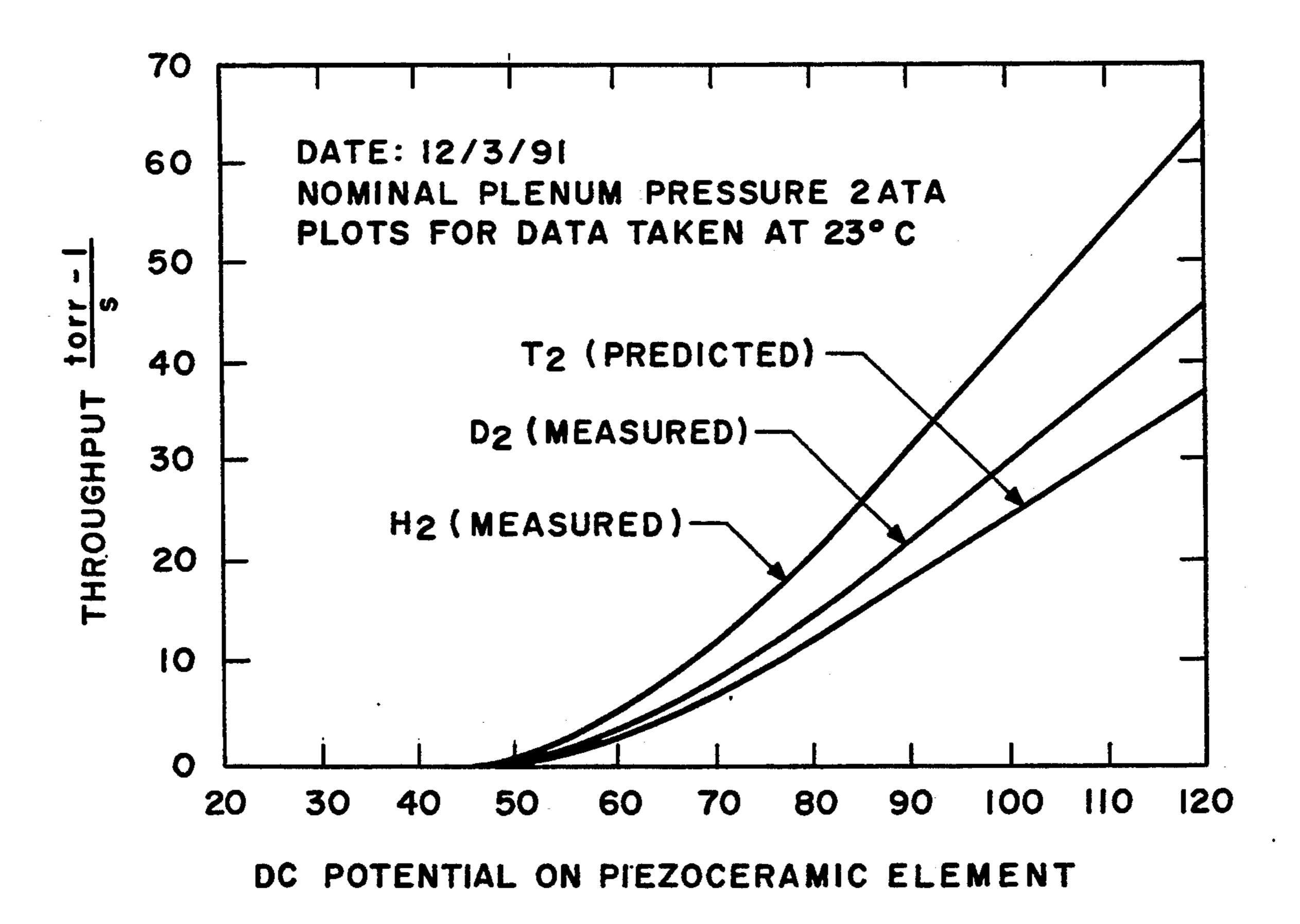
PIEZOELECTRIC VALVE CHARACTERIZATION CURVES
