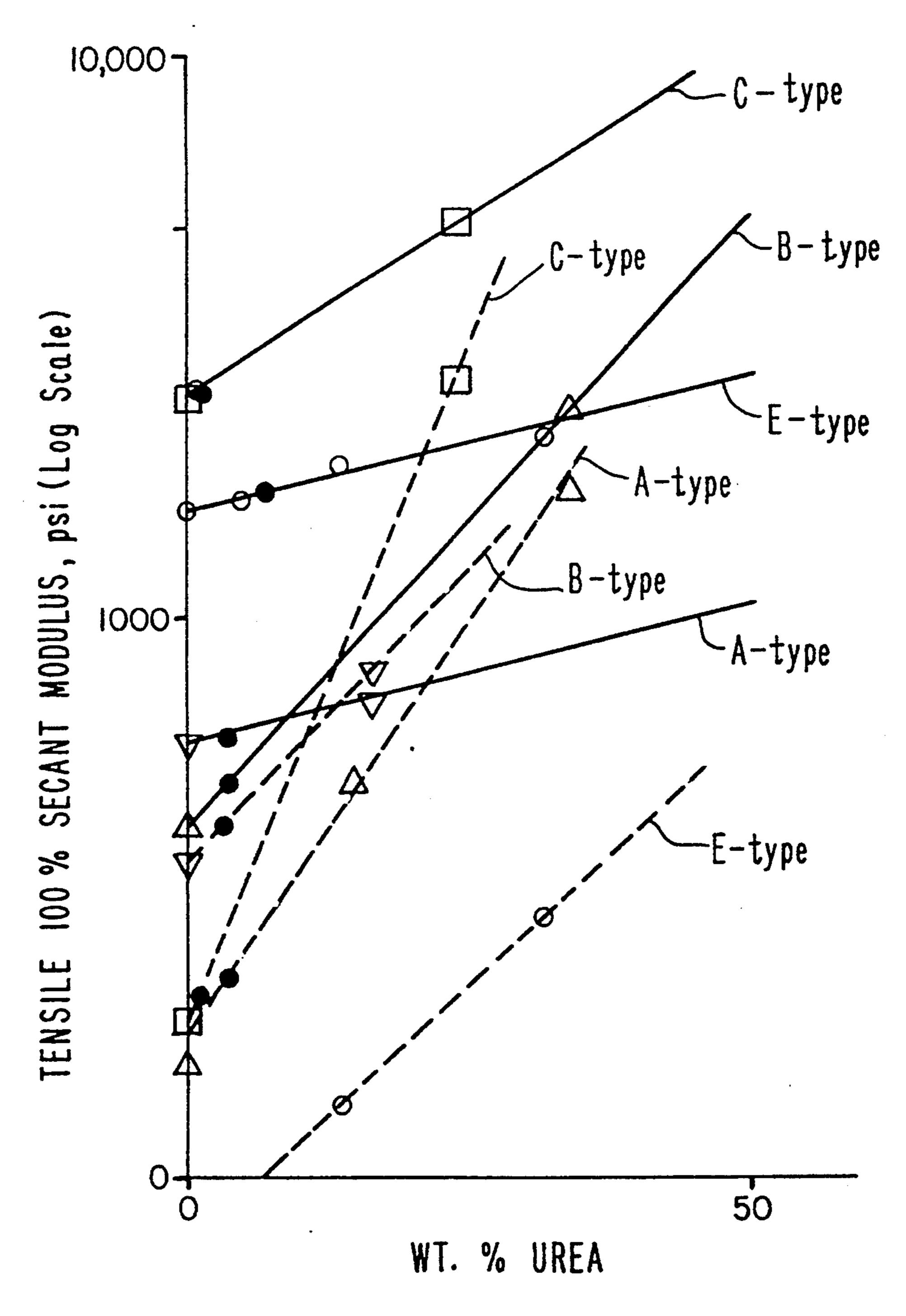
SOLID LINE = DRY POLYMER DASHED LINE = HYDRATED POLYMER
