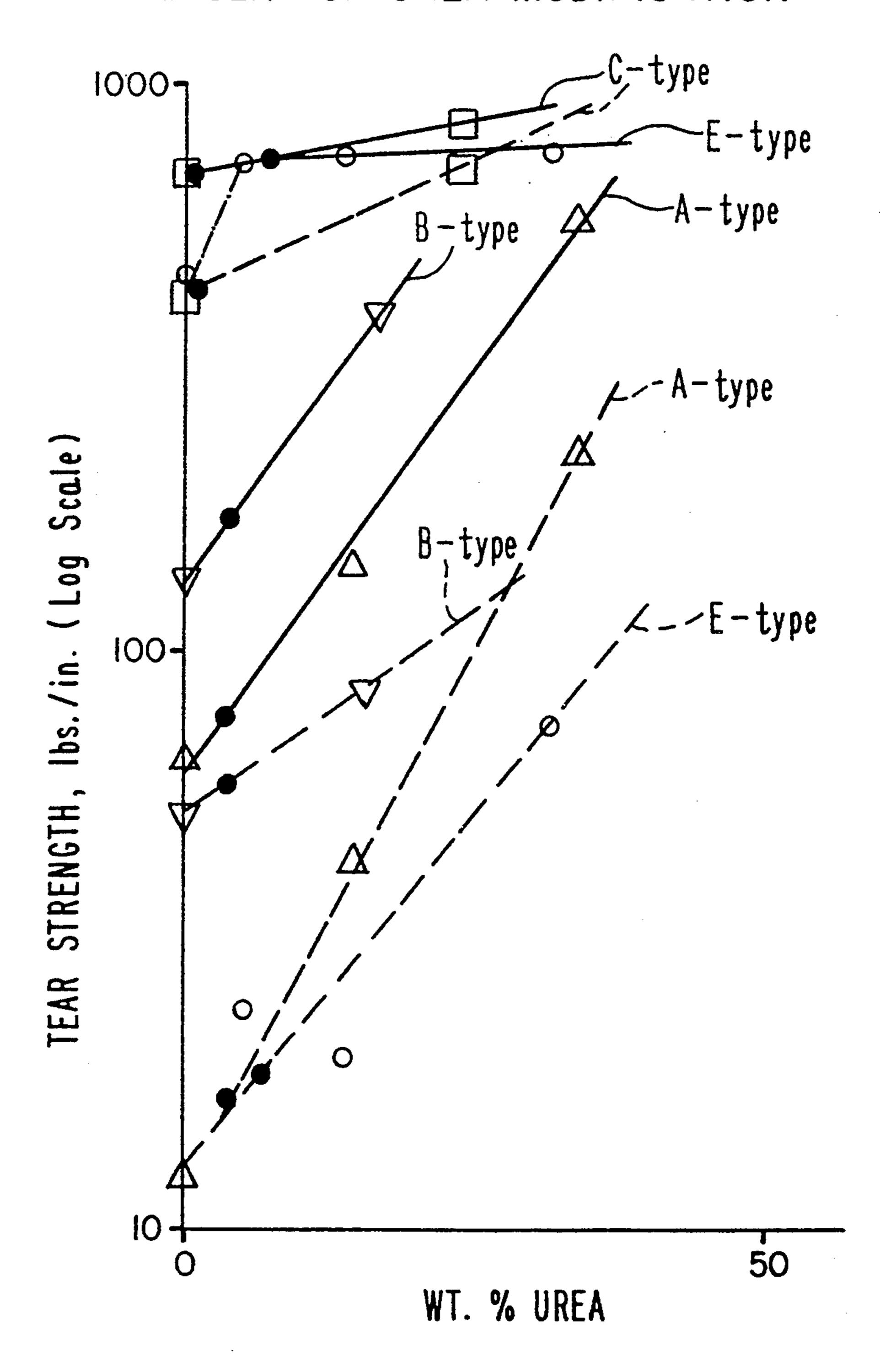
SOLID LINE = DRY POLYMER DASHED LINE = HYDRATED POLYMER
