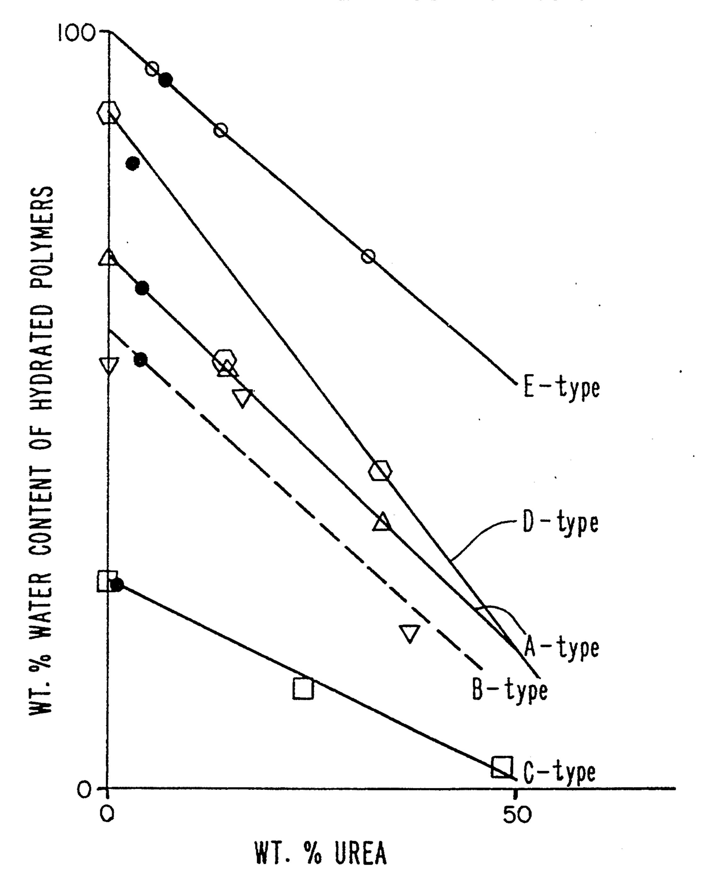
SOLID LINE = DRY POLYMER DASHED LINE = HYDRATED POLYMER
