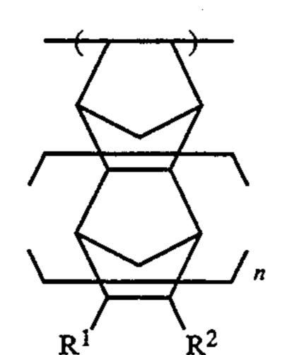
wherein n is 0,  $R^1$  is —CH=CH<sub>2</sub> and  $R^2$  is H; or n is 1,  $R^1$  is =CH—CH<sub>3</sub> and  $R^2$  is H.
