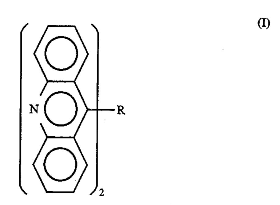
wherein R represents an alkylene, oxadialkylene or thiodialkylene group having 2 to 20 carbon atoms, and a photopolymerizable element comprising a layer of the photopolymerizable composition formed on a support.
