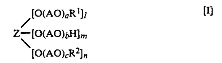
where Z is a residue of a compound having 2-8 hydroxyl groups, AO is an oxyalkylene group having 2-18 carbon atoms,  $R^1$  is an unsaturated hydrocarbon group having 2-5 carbon atoms,  $R^2$  is a hydrocarbon group having 1-40 carbon atoms, a=0 to 1000, b=0 to 1000, c=0 to 1000, l=1 to 8, m=0 to 2, n=0 to 7, (l+m+n)=2 to 8, (al+bm+cn)=1 to 1000,  $m/(l+n) \le \frac{1}{2}$ .
