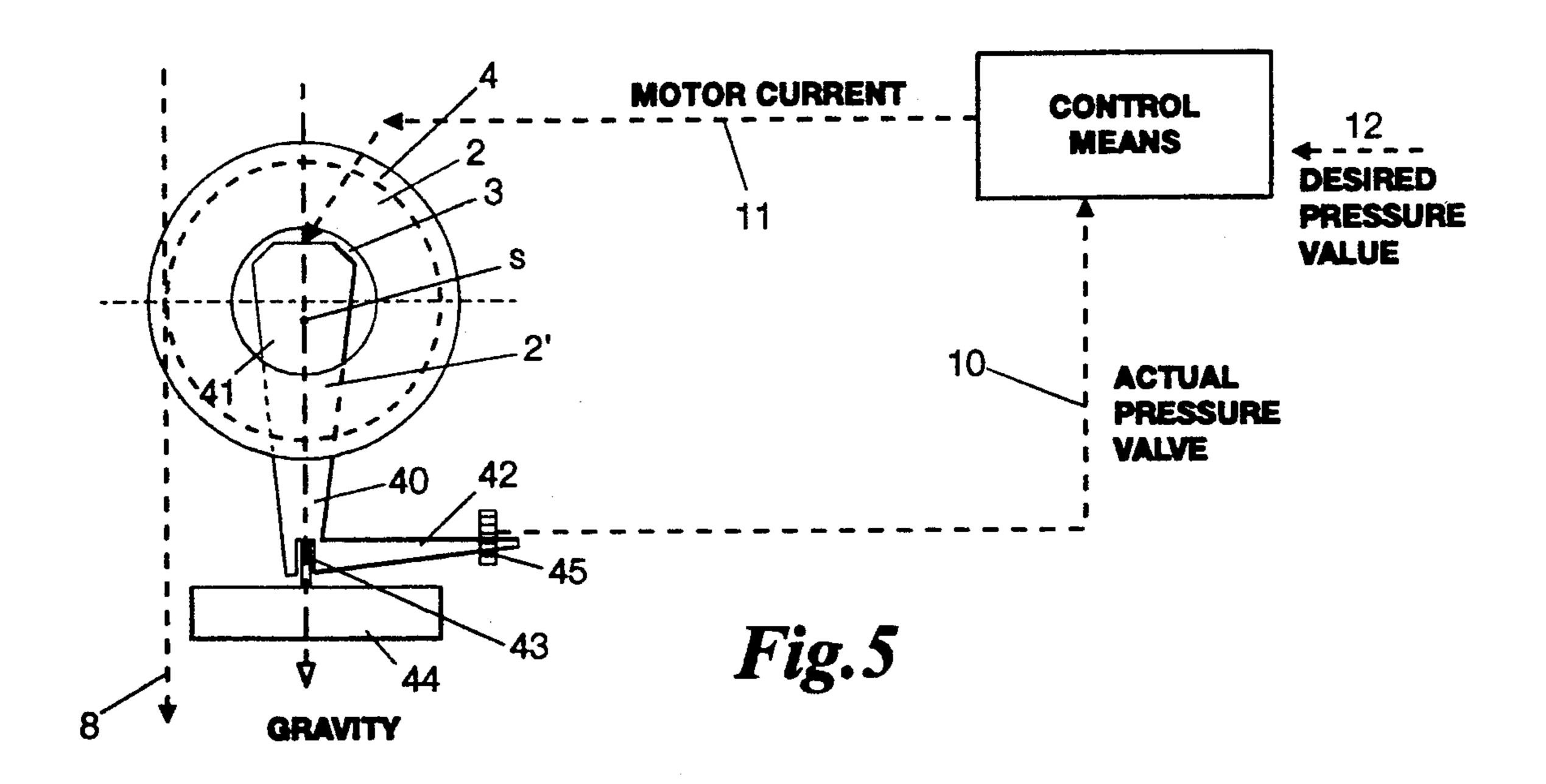
APPARATUS FOR MEASURING AND/OR CONTROLLING THE TENSION IN A RIBBON OR WIRE-TYPE ELECTRODE OF AN ELECTRIC DISCHARGE MACHINE
