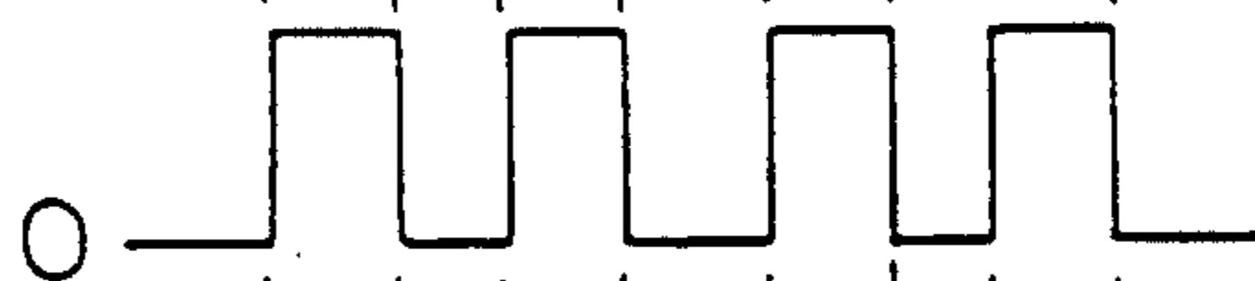
FIG. 16(b) PRIOR ART AMPLITUDE OF LIGHT RIGHT AFTER PASSING THE PHOTOMASK
