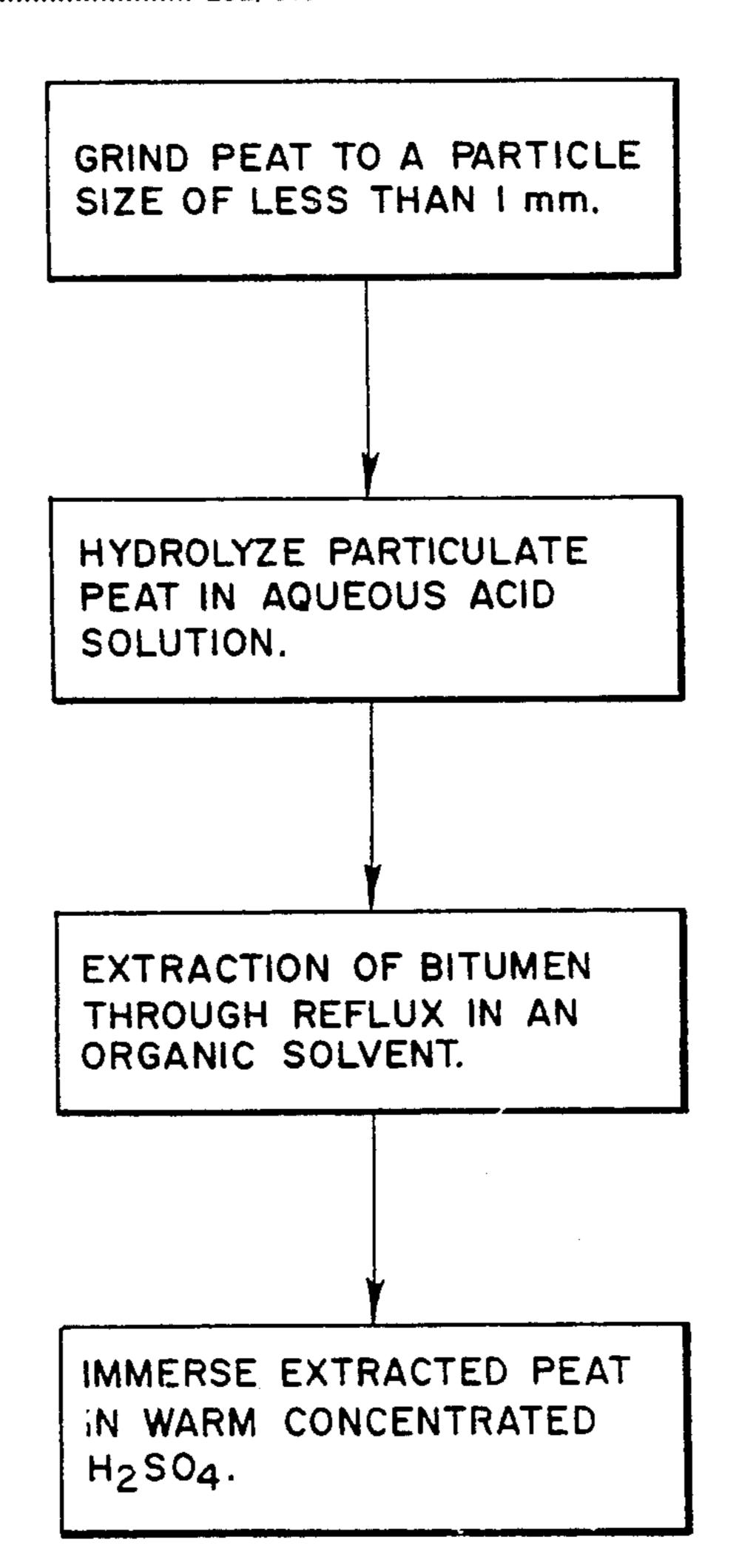
SIZE OF LESS THAN I mm. HYDROLYZE PARTICULATE PEAT IN AQUEOUS ACID SOLUTION. EXTRACTION OF BITUMEN THROUGH REFLUX IN AN ORGANIC SOLVENT. IMMERSE EXTRACTED PEAT IN WARM CONCENTRATED
