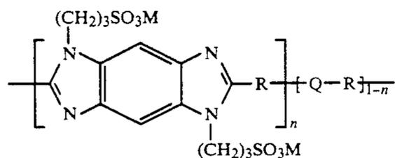
wherein n has a value of 0.05 to 1.00, M is an alkali metal such as Na, Q is a benzobisazole of the formula
