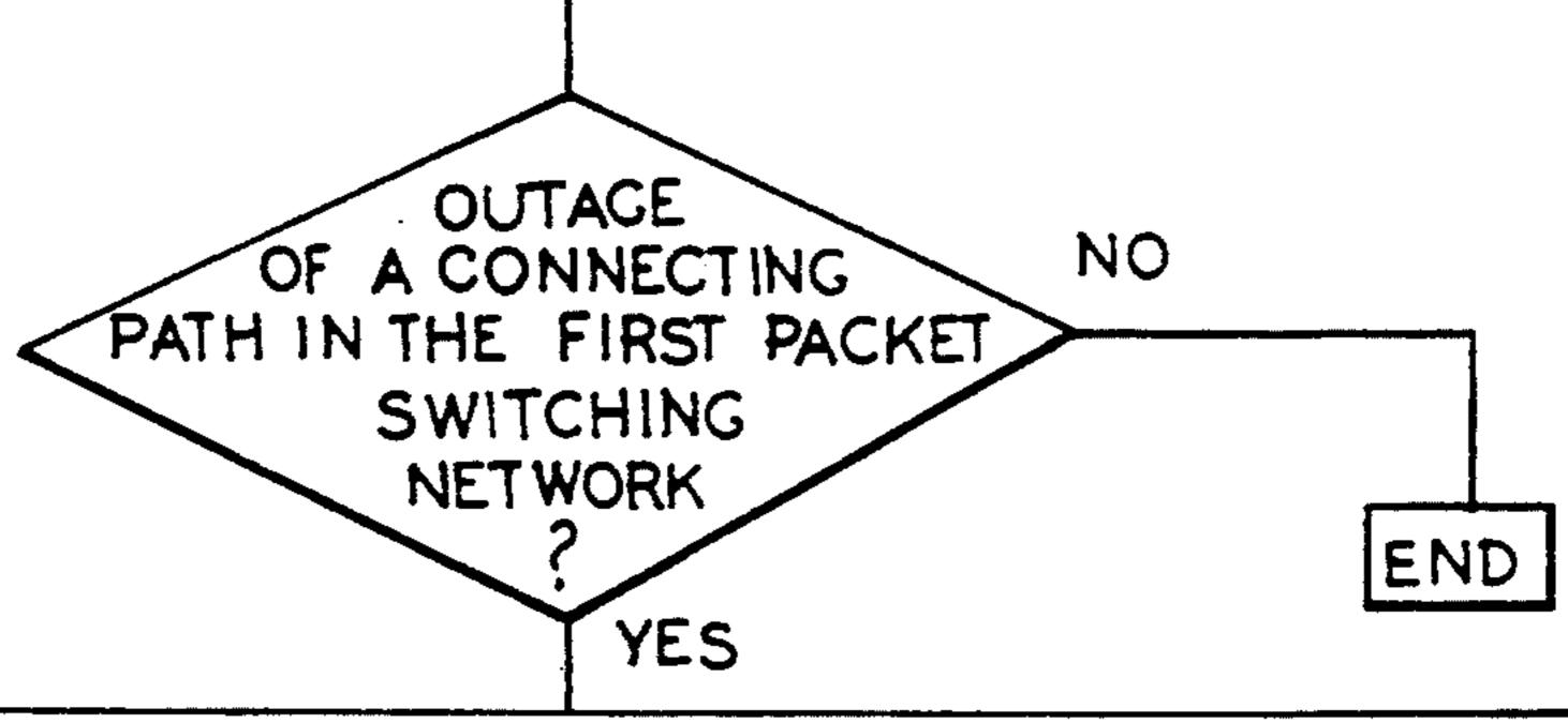
CLEARING DOWN A VIRTUAL CONNECTION CONDUCTED OVER THE CONNECTING PATH TO THE SWITCHING EQUIPMENTS CONNECTED TO THE CALLING AND CALLED SUBSCRIBER EQUIPMENTS PARTICIPATING IN THAT VIRTUAL CONNECTION
