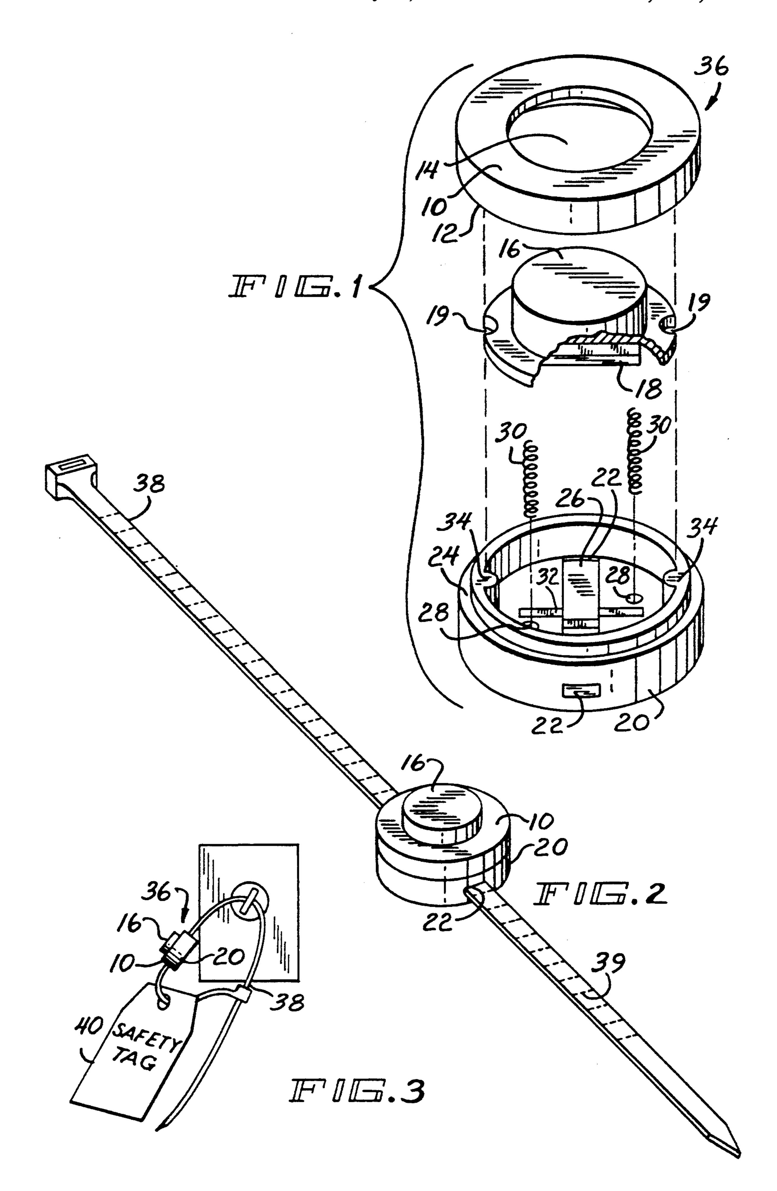
FIG. 3 is a perspective view showing the present invention positioned on a tie wrap that has been secured for its intended use.
