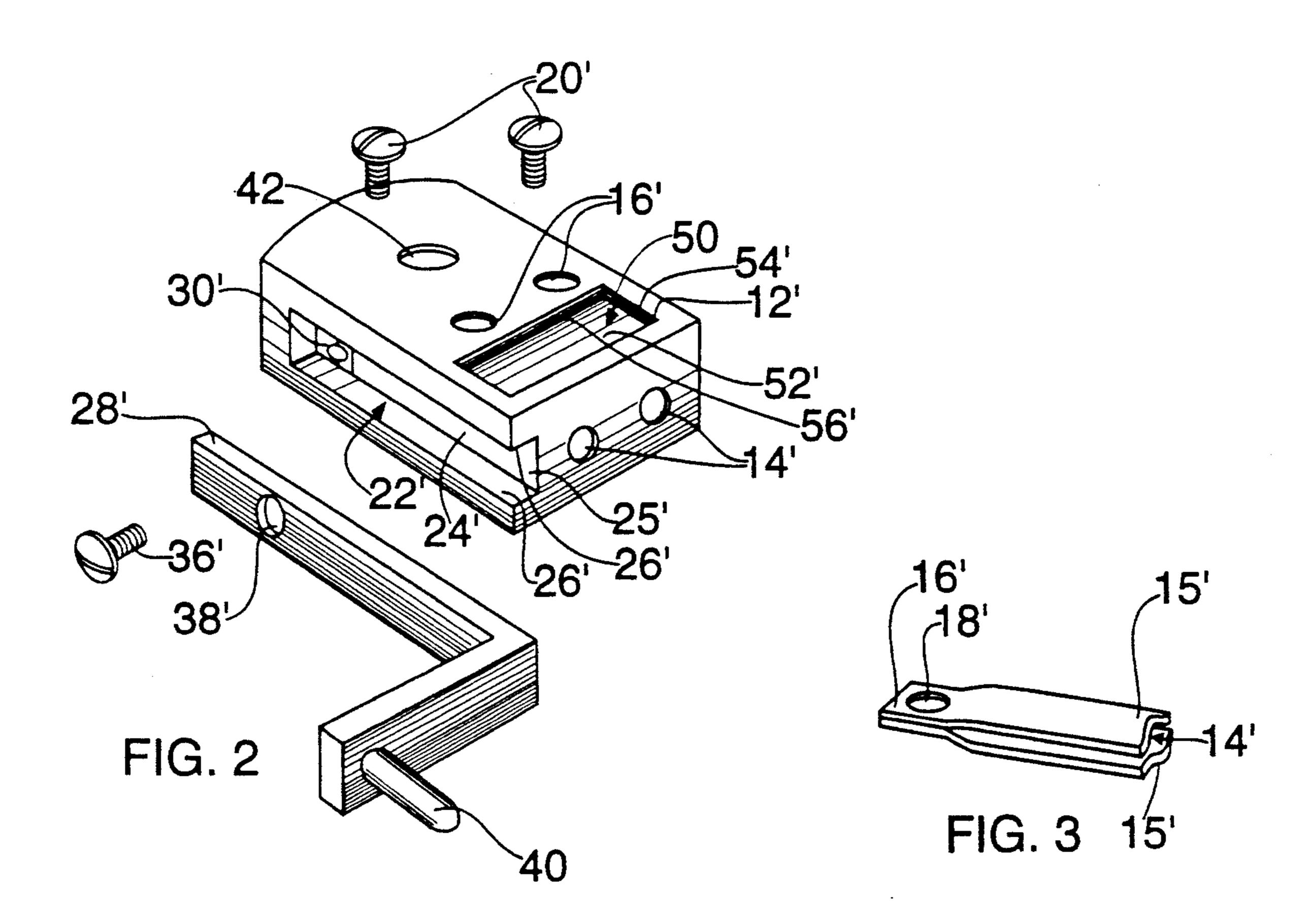
ELECTRICAL CONNECTOR WITH ADAPTABLE EXTERNAL GROUND AND INDICIA DISPLAY
