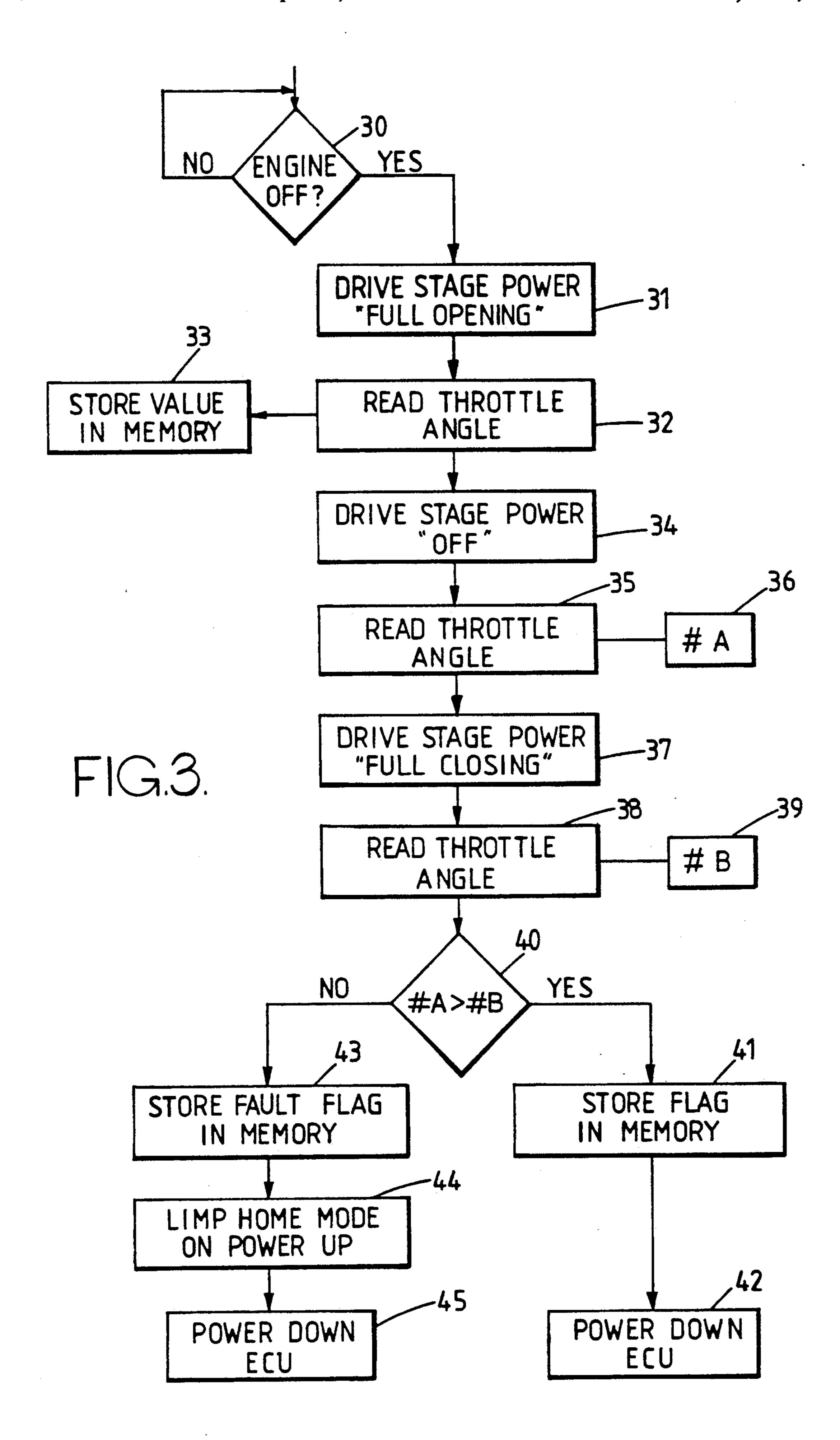
The return system may comprise a closing system, for instance a throttle closing system suitable for use with a throttle of an internal combustion engine.
