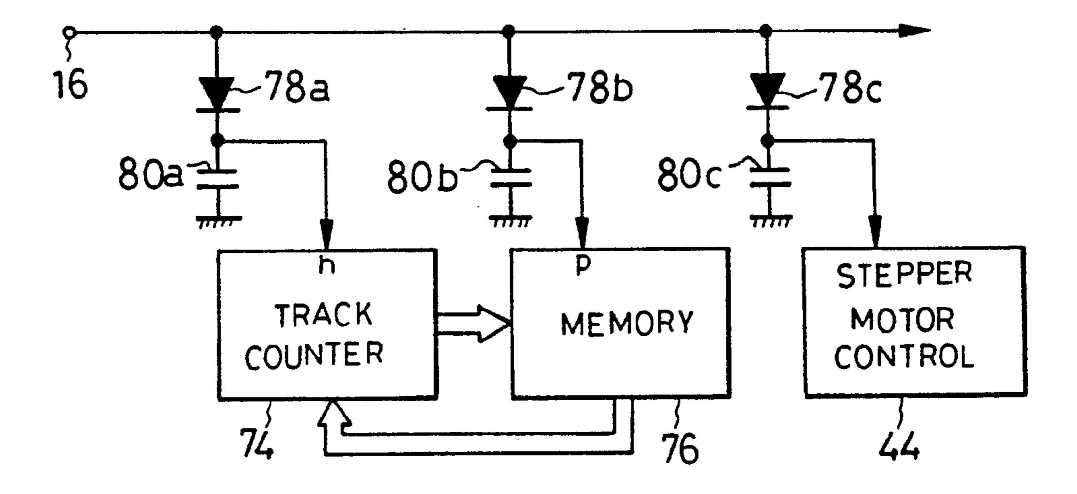
SYSTEM FOR HOLDING A TRACK COUNTER **ACTIVE DESPITE POWER SUSPENSION IN** ROTATING DISK DATA STORAGE APPARATUS
