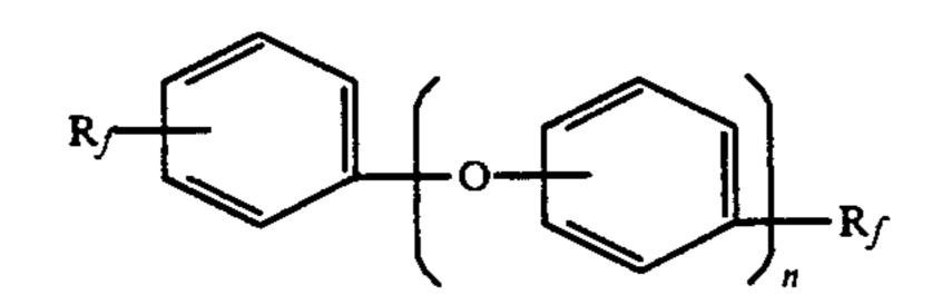
where R<sub>f</sub> is a perfluoroalkyl group having 1 to 15 carbon atoms and n has a value of 1 to 6, for perfluoropolyalkylether fluids. These additives are incorporated into perfluoropolyalkylether fluids in an amount ranging from about 0.01 to 3 weight percent.
