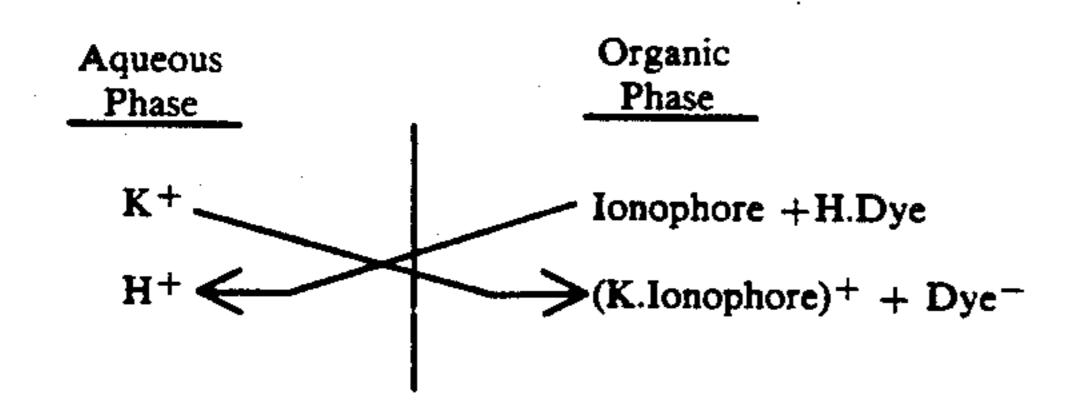
The degree and intensity of the color transition due to the above reaction is proportional to the amount of potassium ion in the test sample and is monitored by reflectance spectroscopy at 640 nm with reflectance measurements taken at five second intervals. Results 20 can be displayed digitally by an instrument in units of mMol/L.
