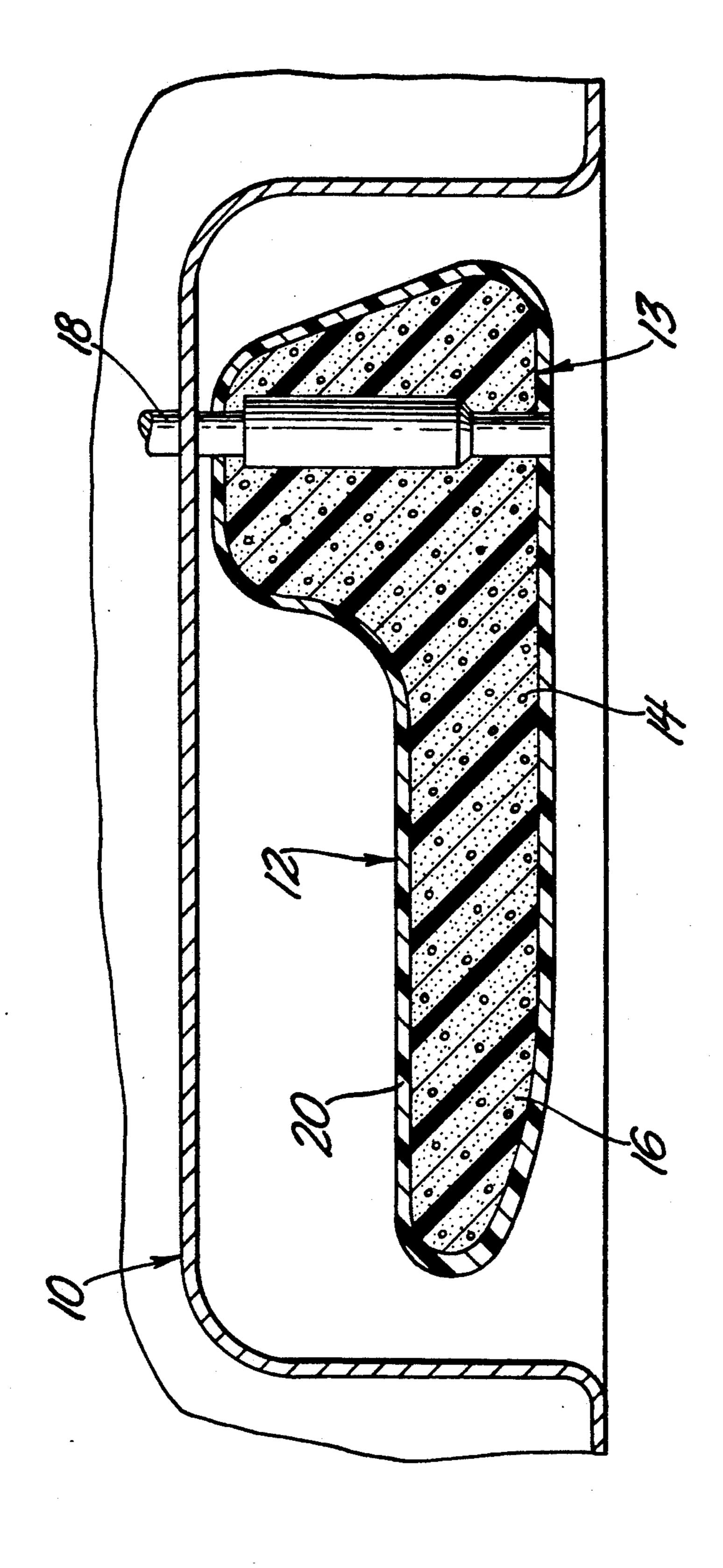
In addition, the outer skin layer has a thickness in the range of 0.2 to 2.0 millimeters.
