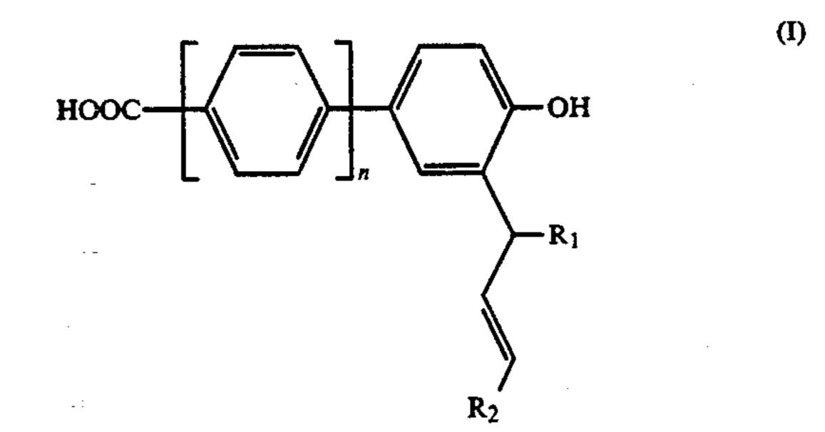
is disclosed, which consists of a first step of simultaneous esterification and etherification of a carboxylated phenol, subsequent rearrangement of the resulting product to yield allyl-carboxylated allyl-phenol and end saponification of the latter into carboxylated 2-allylphenol.
