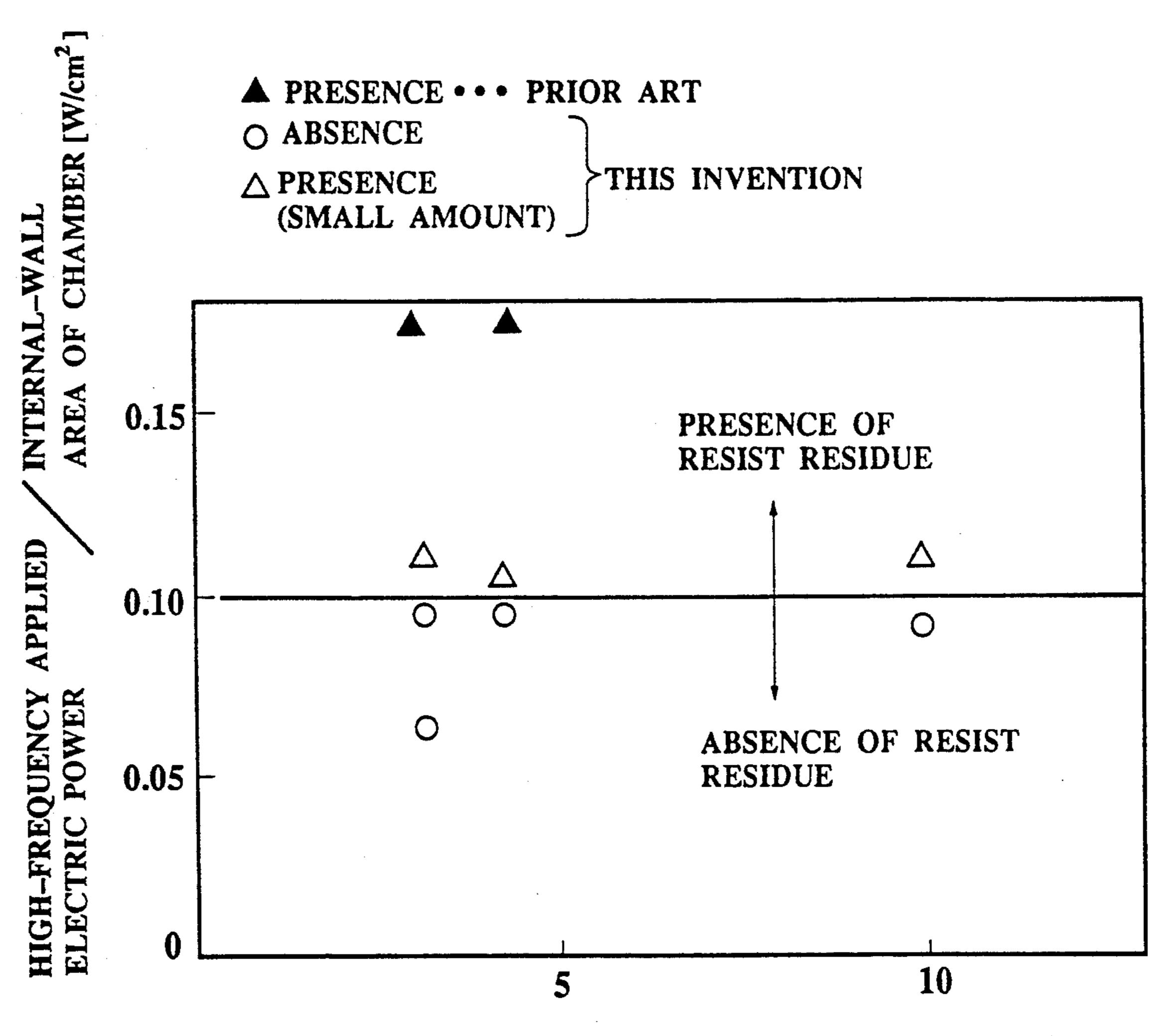
INTERNAL-WALL AREA OF CHAMBER [×10<sup>3</sup> cm<sup>2</sup>]
