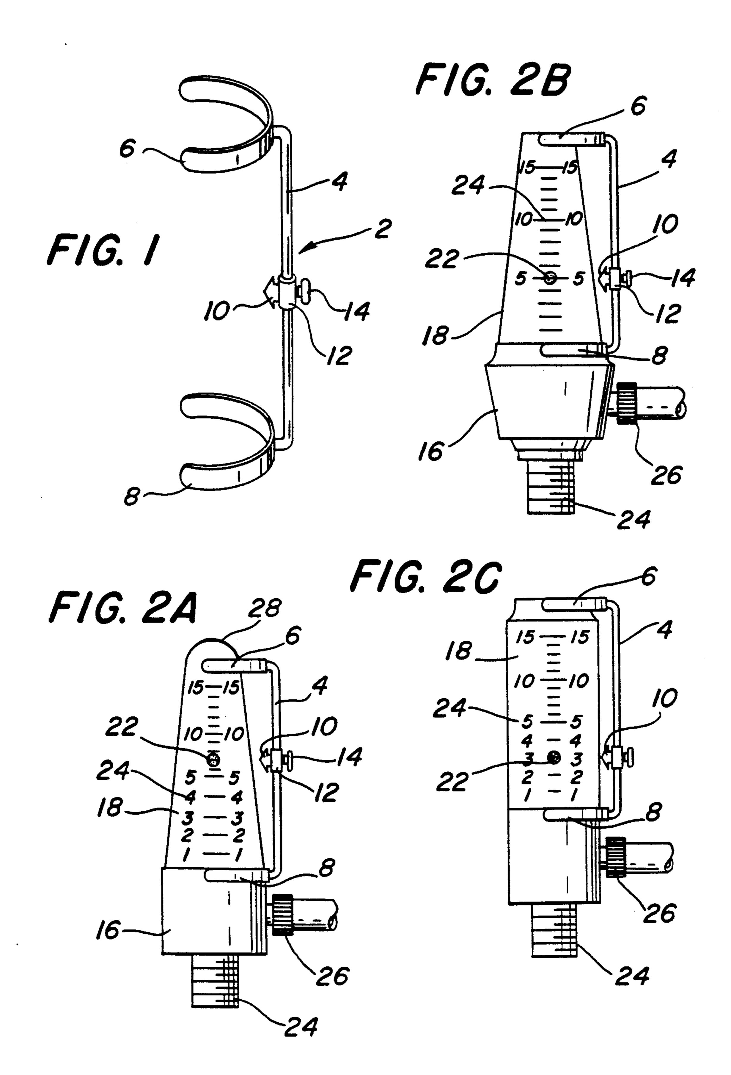
annular ring surrounding the rod which can be moved longitudinally along the rod to a pre-determined level of oxygen flow.
