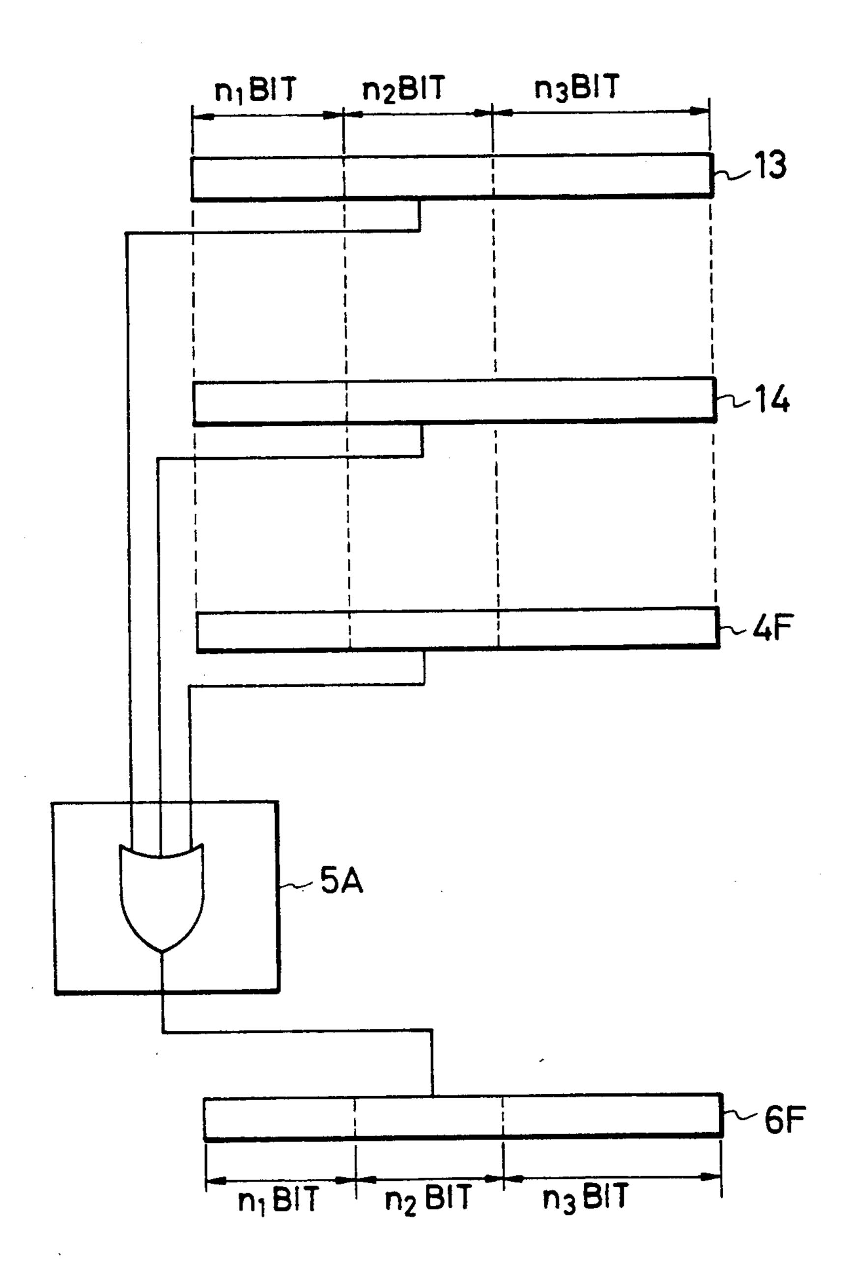
DATA PROCESSING SYSTEM HAVING A PLURALITY OF REGISTER GROUPS AND A LOGICAL OR CIRCUIT FOR ADDRESSING ONE REGISTER OF ONE OF THE REGISTER GROUPS
