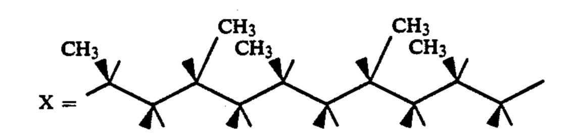
Corresponding representations for syndiotactic polyvinylchloride and polystyrene respectively are:
