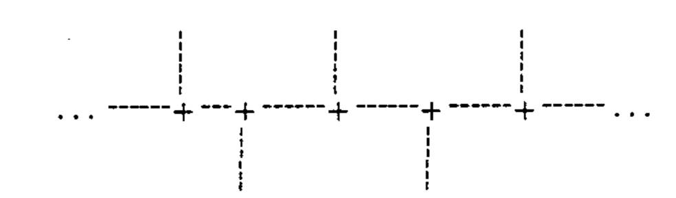
In NMR nomenclature, this pentad is described as ... rrrr... in which each "r" represents a "racemic" dyad, i.e., successive methyl groups on alternate sides of the plane. The percentage of r dyads in the chain determines the degree of syndiotacticity of the polymer.
