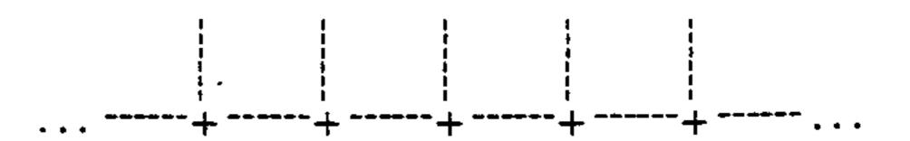
Another way of describing the structure is through the use of NMR. Bovey's NMR nomenclature for an isotactic pentad is ... mmmm... with each "m" representing a "meso" dyad or successive methyl groups on the same side in the plane. As known in the art, any deviation or inversion in the structure of the chain lowers the degree of isotacticity and crystallinity of the polymer.
