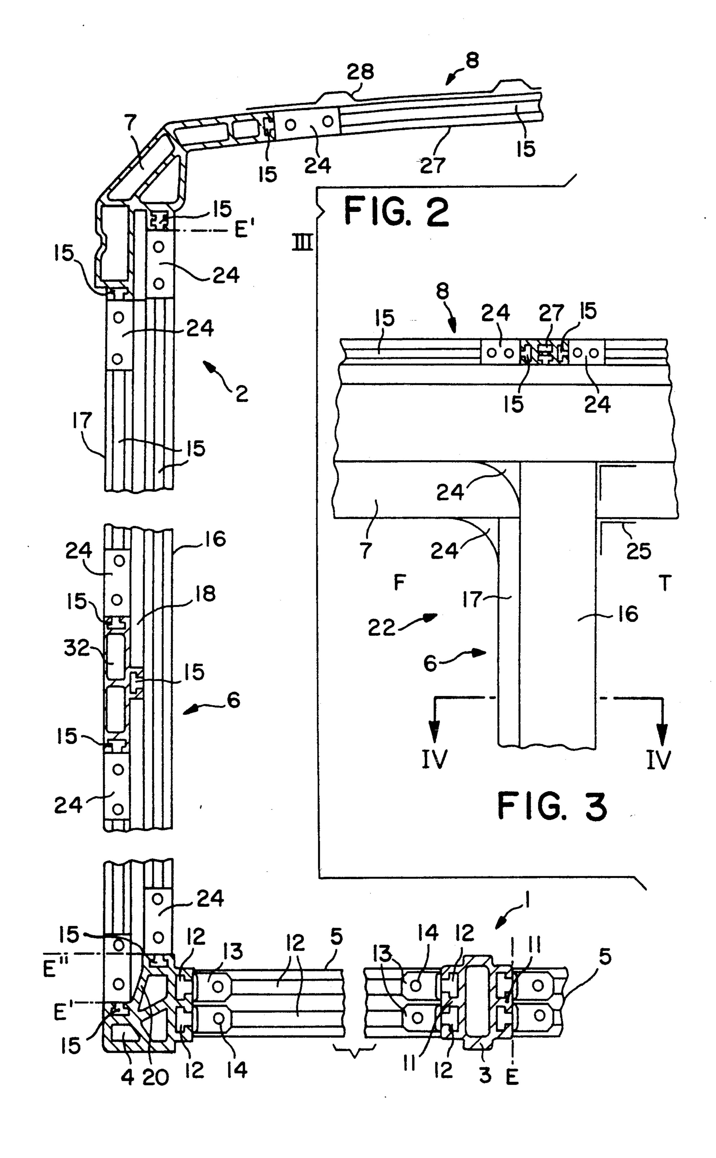
COACH BODY CONSTRUCTION FOR RAIL VEHICLES HAVING EXTRUDED ALUMINUM PROFILES WITH UNDERCUT NUT-RECEIVING GROOVES FOR EASE OF ASSSEMBLY
