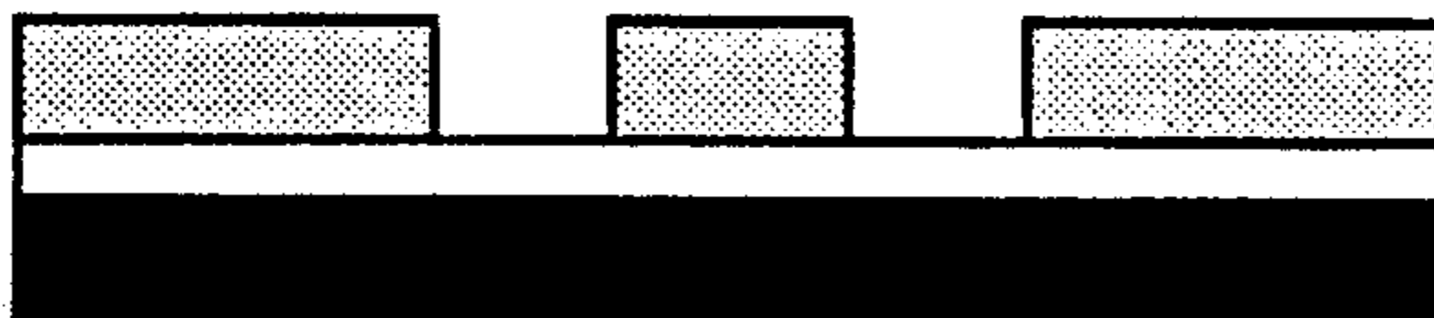
Fig. 4b. The photoresist is exposed and developed.
