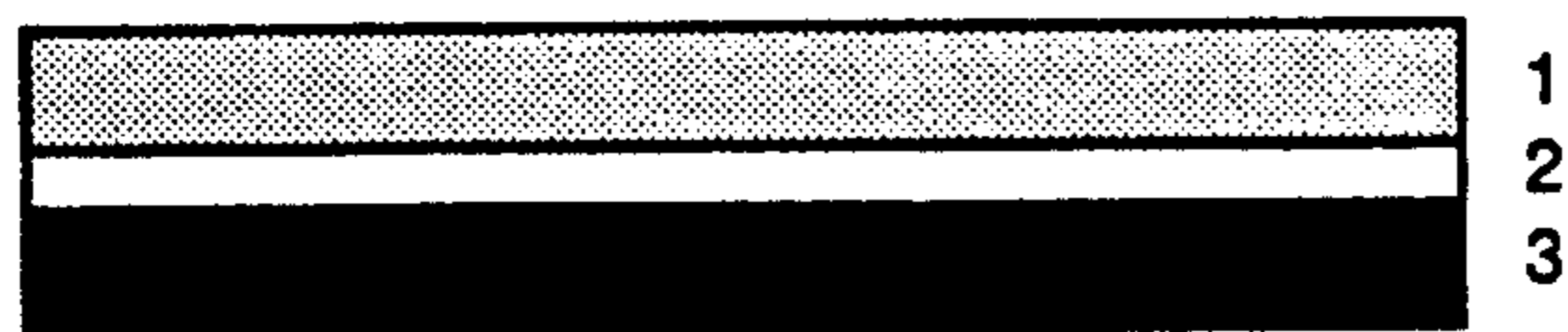
Fig. 9a. A bilvel resist structure comprised of photoresist over a wet-developable release layer.
