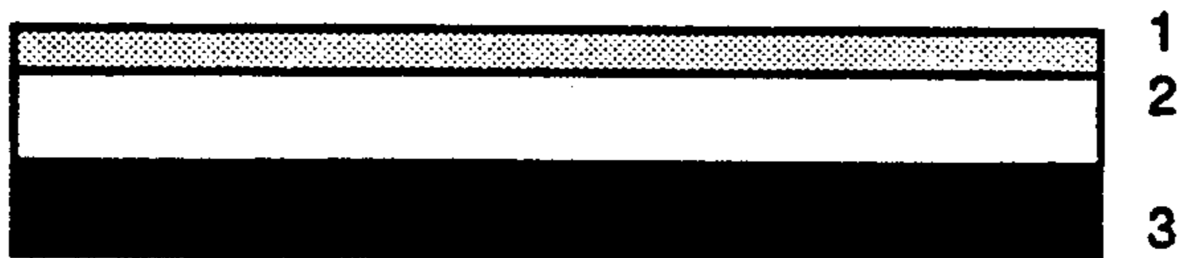
Fig. 10a. A bilayer resist structure comprised of photoresist over wet-developable release layer.
