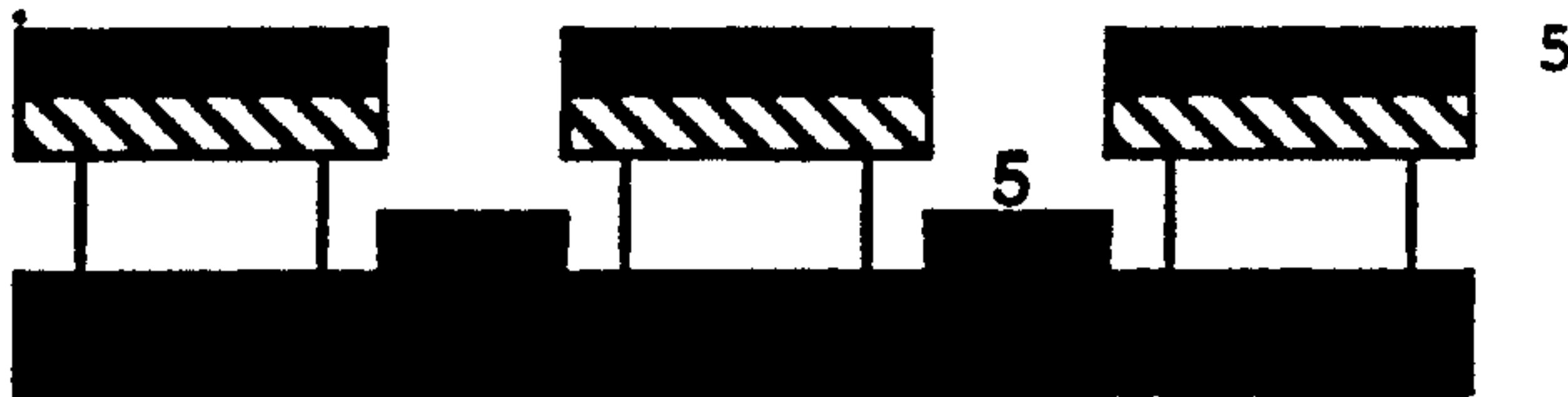
Fig. 1e. Metal is deposited on the specimen by evaporation or sputtering through the metal/glass-release layer mask.
