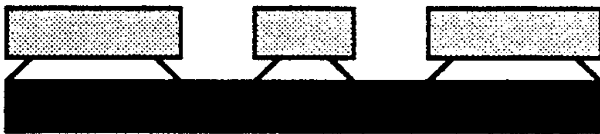
Fig. 8b. The photoresist and release layer are developed in dilute aqueous base, producing features with non-vertical walls in the release layer level.
