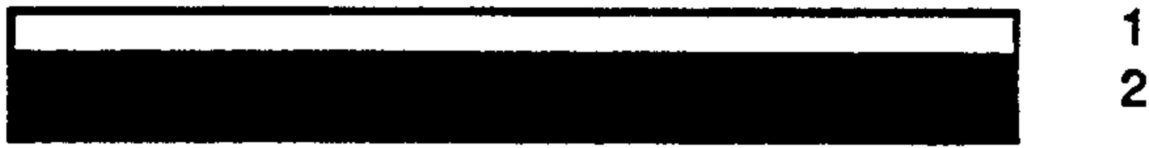
Fig. 5a. A release layer film is spincoated on the substrate and baked to remove solvents.
