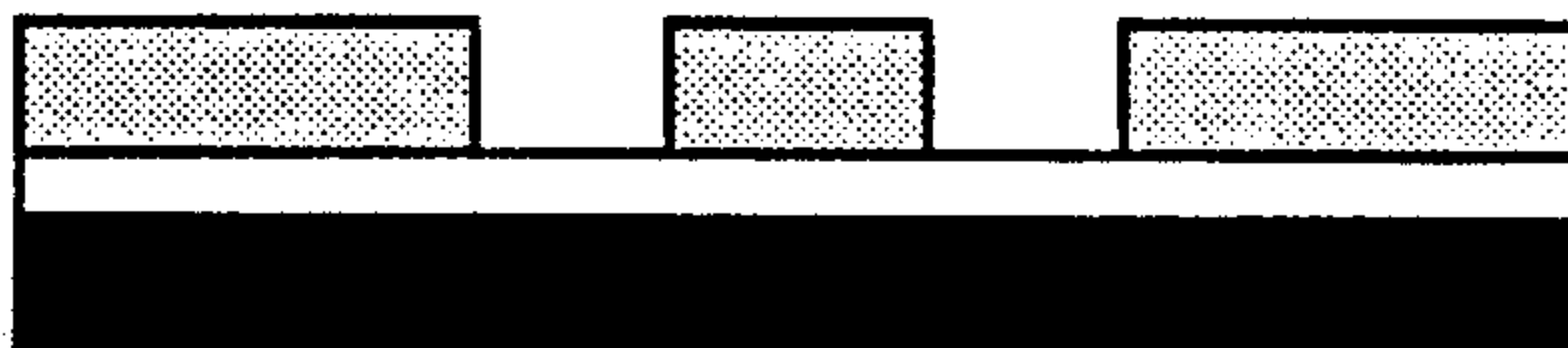
Fig. 4b. The photoresist is exposed and developed.
