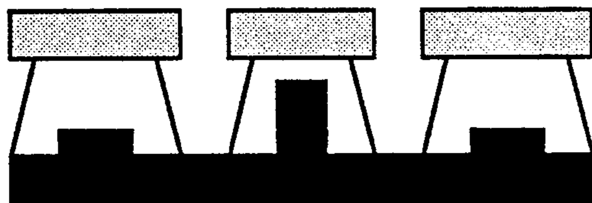
Fig. 11b. The photoresist and release layer are developed in dilute aqueous base, producing features with non-vertical walls in the release layer level.
