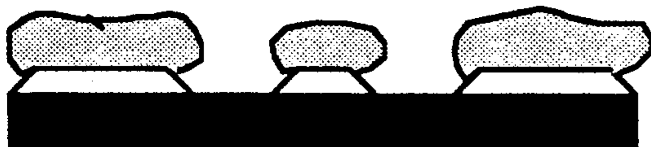
Fig. 8d. The structure is baked at temperatures >150^{\circ} causing photoresist deformation and converting the photoresist to a chemically intractable form.
