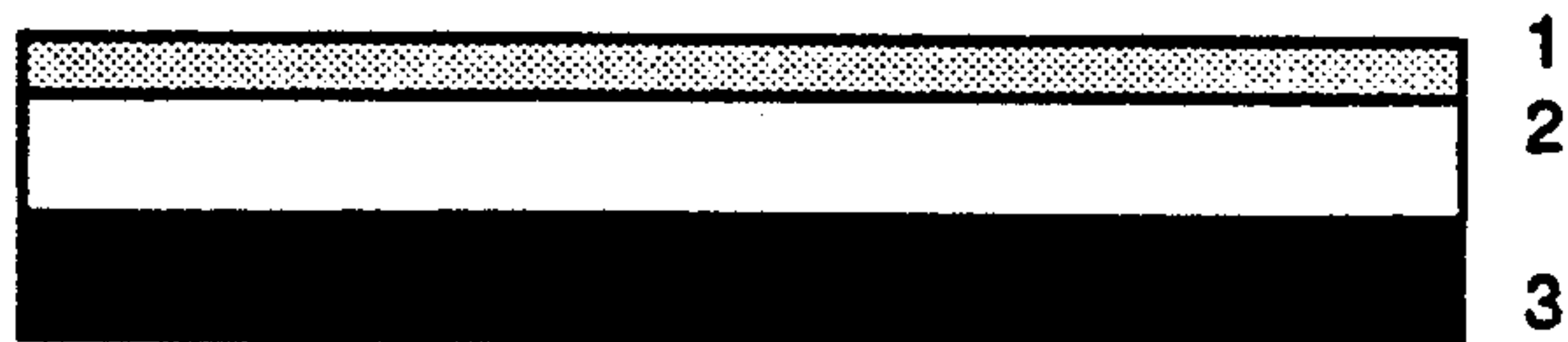
Fig. 10a. A bilvel resist structure comprised of photoresist over wet-developable release layer.
