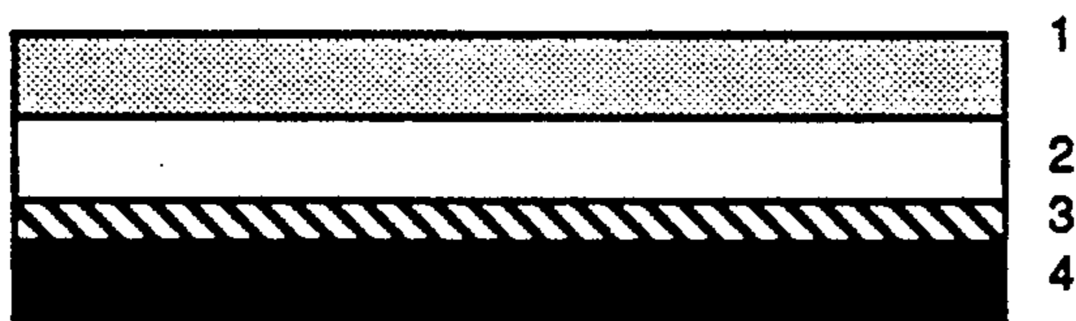
Fig. 3a. A multilevel resist structure for dry etch patterning of a metal layer.
