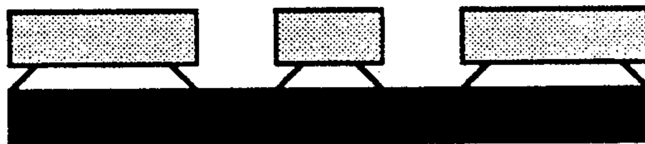
Fig. 9b. The photoresist and release layer are developed in dilute aqueous base, producing features with non-vertical walls in the release layer level.
