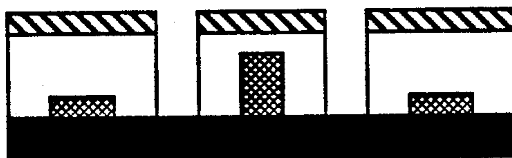
Fig. 2d. Oxygen reactive ion etching is then applied to transfer the photoresist pattern into the release layer anisotropically; the photoresist is removed at the same time.
