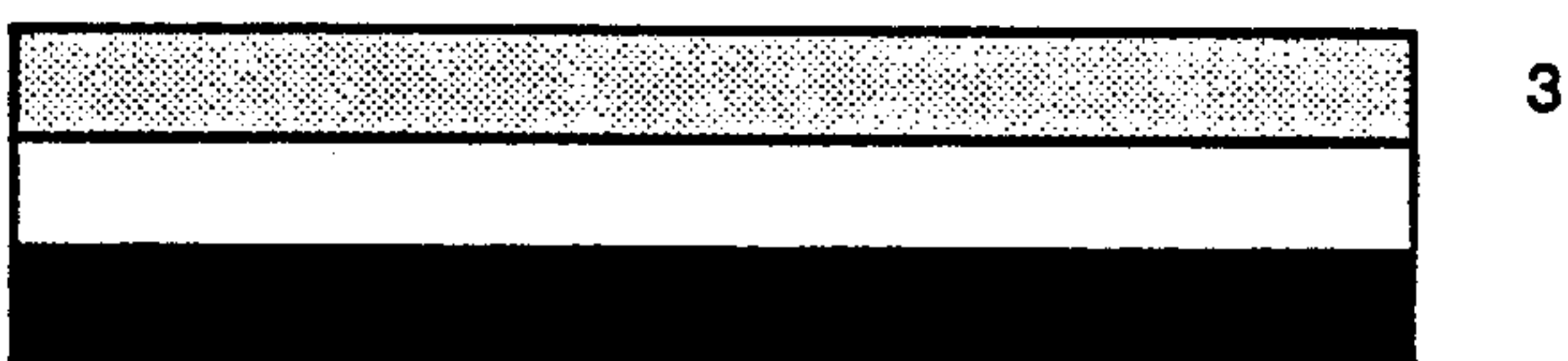
Fig. 6b. Positive photoresist is applied over the polyamic acid film and soft baked.
