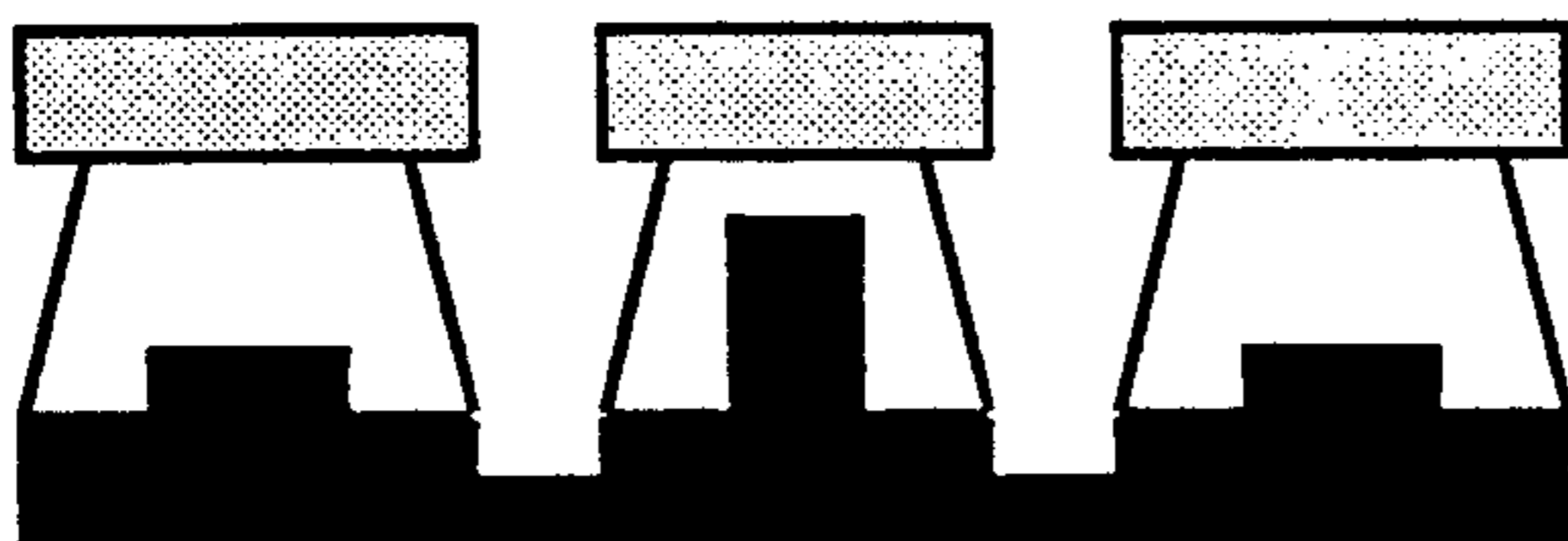
Fig. 11c. The photoresist pattern is transferred into the substrate by reactive ion etching through the photoresist-release layer mask.
