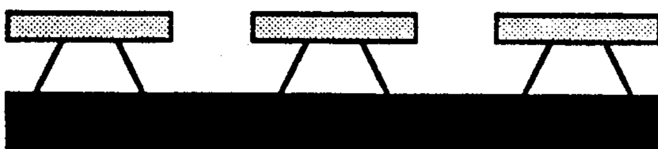
Fig. 10b. The photoresist and release layer are developed in dilute aqueous base, producing features with non-vertical walls in the release layer level.
