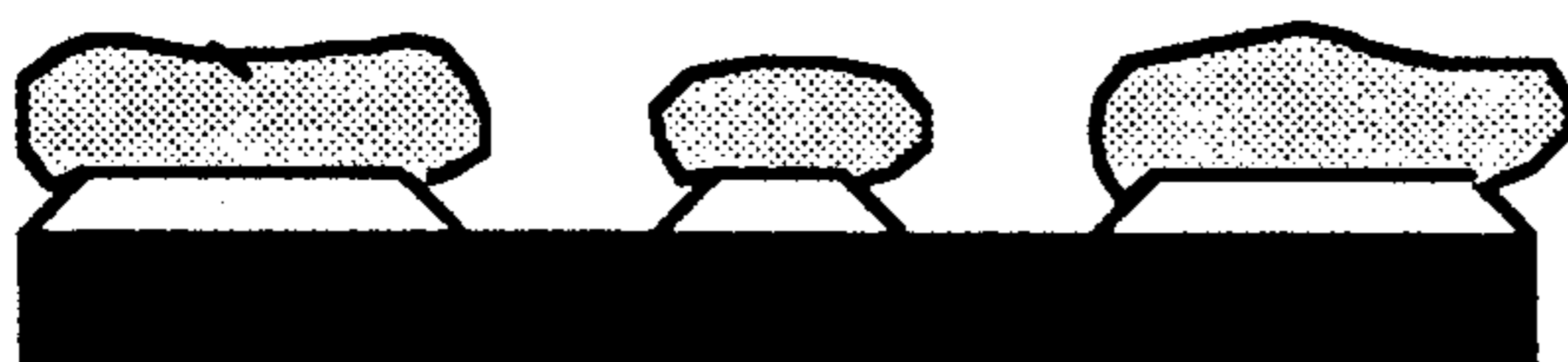
Fig. 8d. The structure is baked at temperatures >150° causing photoresist deformation and converting the photoresist to a chemically intractable form.
