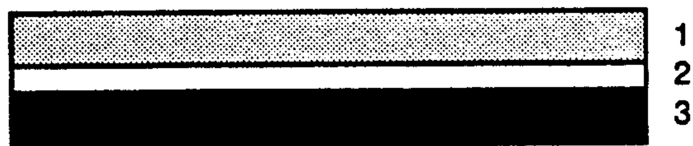
Fig. 9a. A bilayer resist structure comprised of photoresist over a wet-developable release layer.
