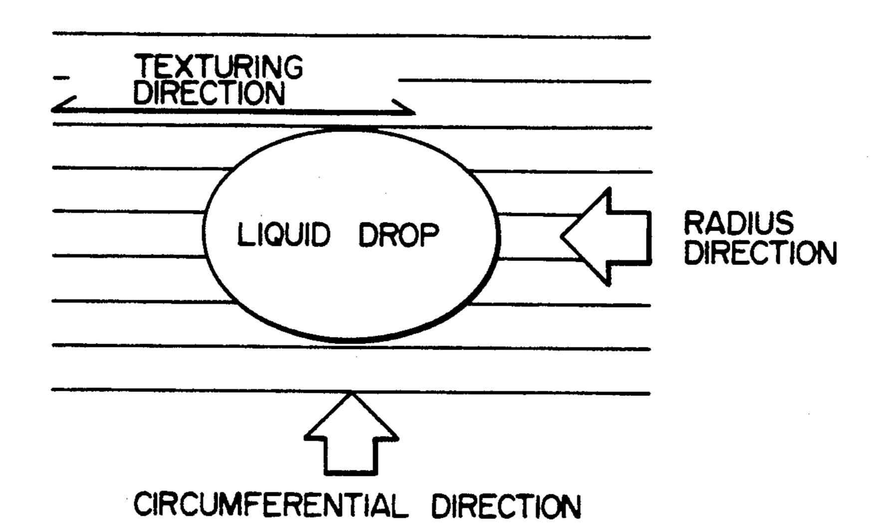
CONTACT ANGLE MEASURING DIRECTION
