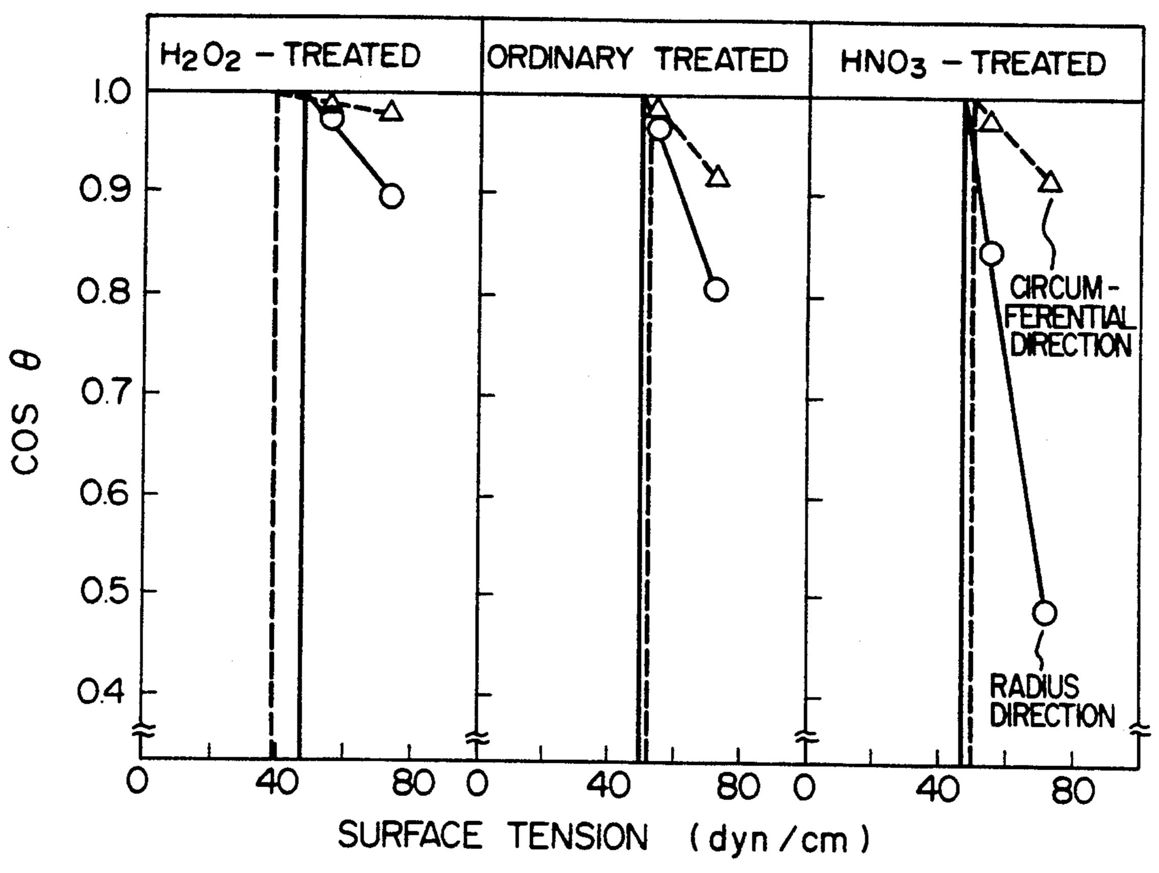
CONTACT ANGLE OF SUBSTRATE (CRITICAL SURFACE TENSION)
