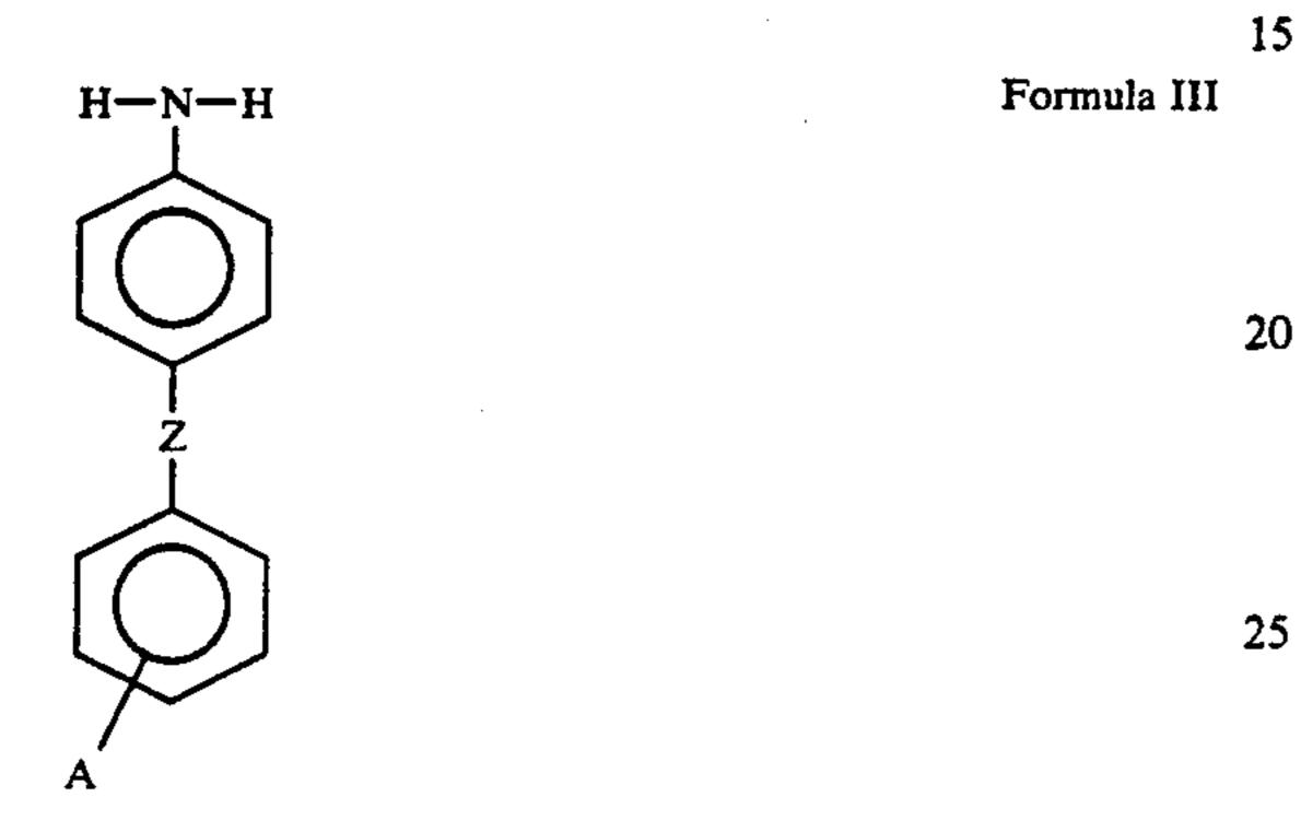
where A is an electron-withdrawing group as described above and Z is an unsaturated bridge between the aromatic rings. The unsaturated bridge between the aromatic rings represented by Z in the above Formula III can be for example, an azo such as -N=N- or any olefinic group such as -CH=CH-.
