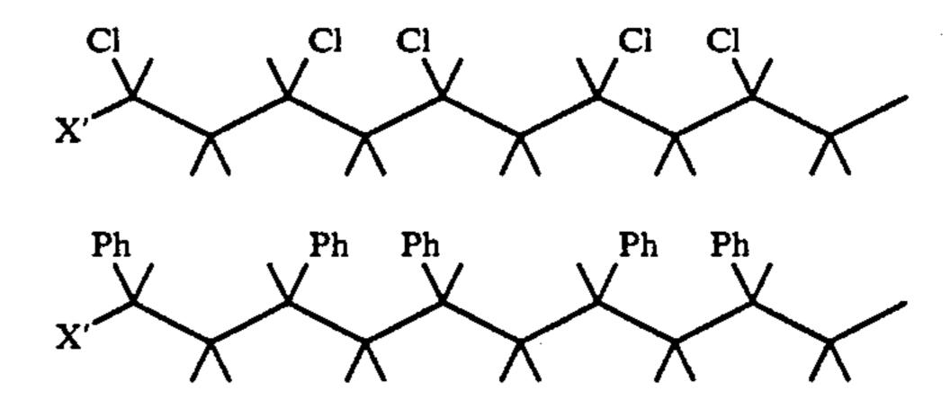
Using the Fischer projection formula, the structure of a syndiotactic polymer or polymer block for polypropylene is designated as:
