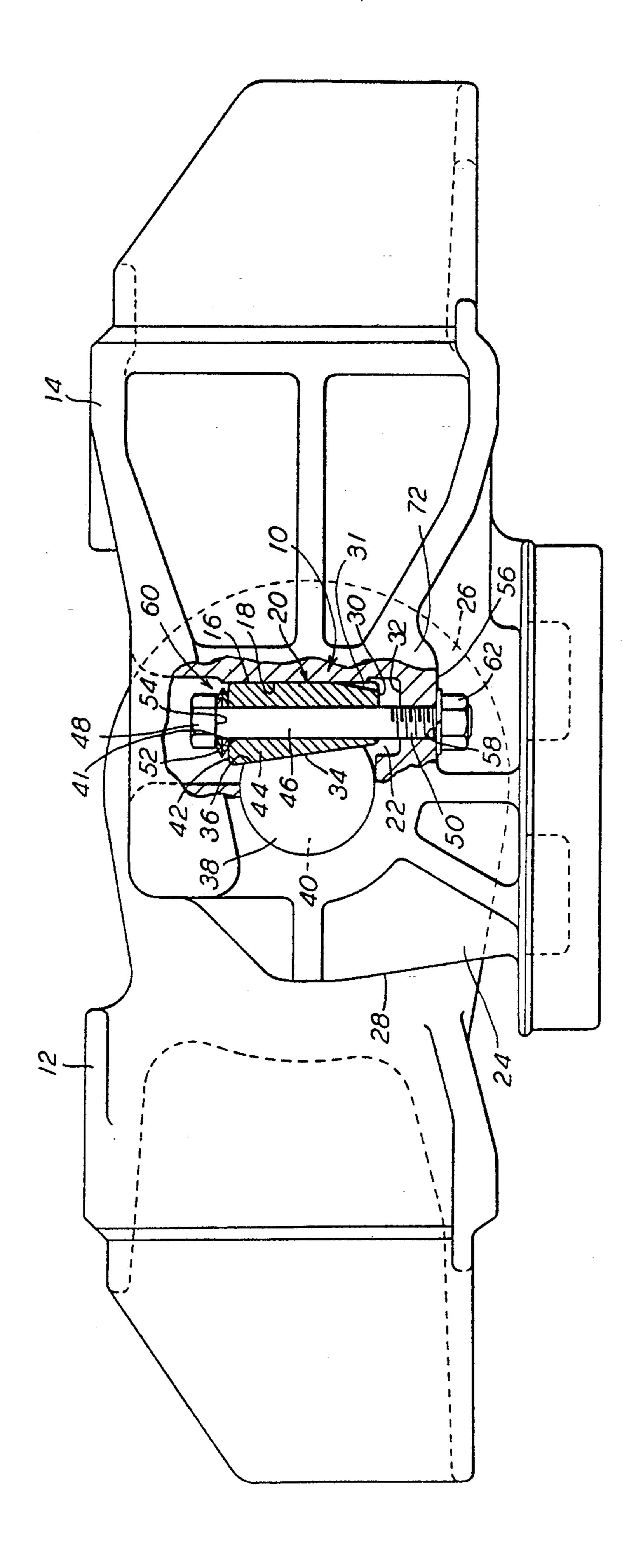
LOCKING WEDGE ASSEMBLY TO REMOVABLY SECURE A MALE CONNECTION MEMBER IN AN ARTICULATED-TYPE COUPLING ARRANGEMENT
