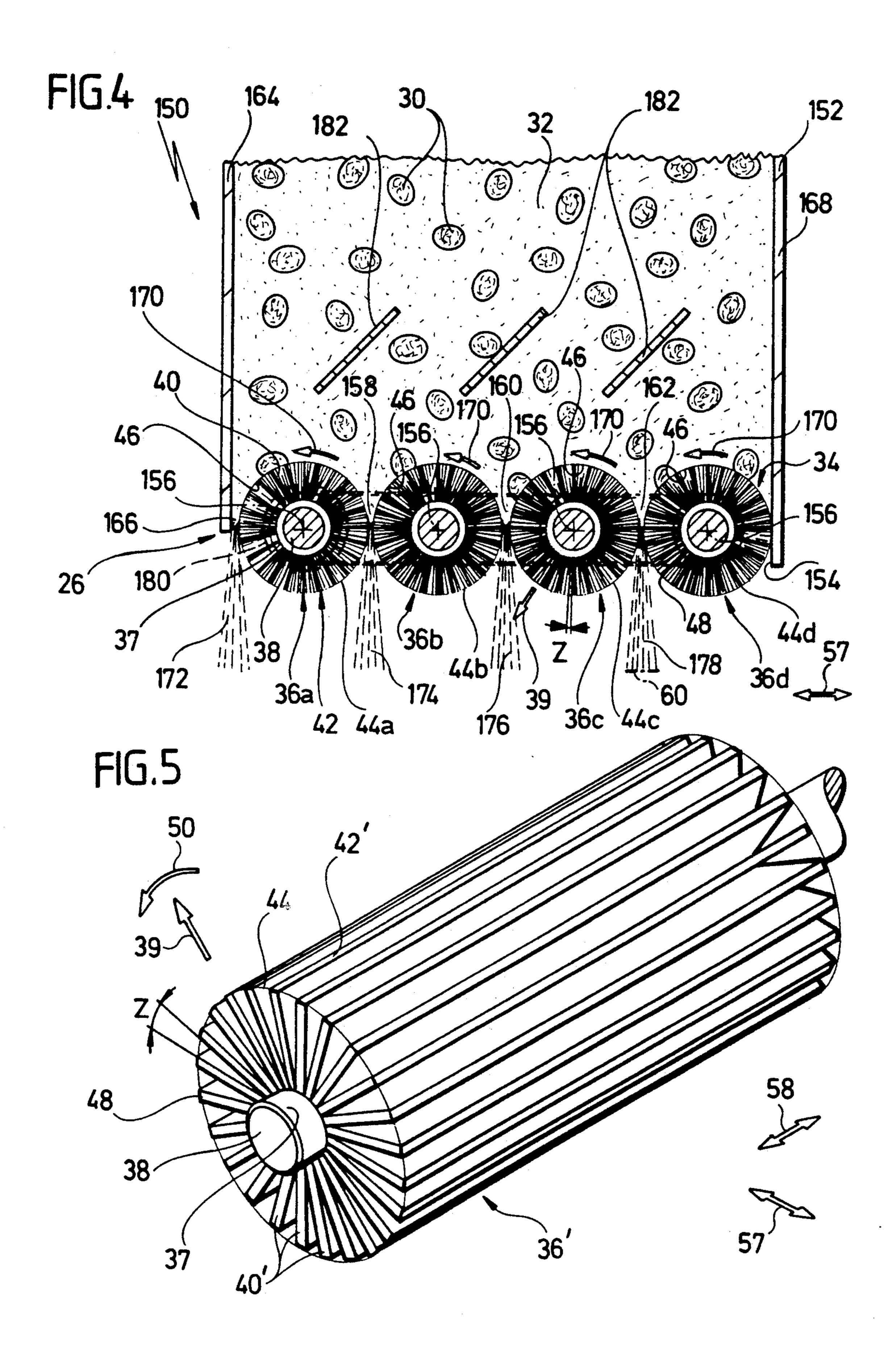
METHOD AND APPARATUS FOR PRODUCING FINELY PULVERIZED SAND PARTICLES FOR USE IN THE PRODUCTION OF CASTING MOLDS AND FOR COATING WITH THE FINELY PULVERIZED SAND PARTICLES MODELS FOR SHAPED CASTINGS
