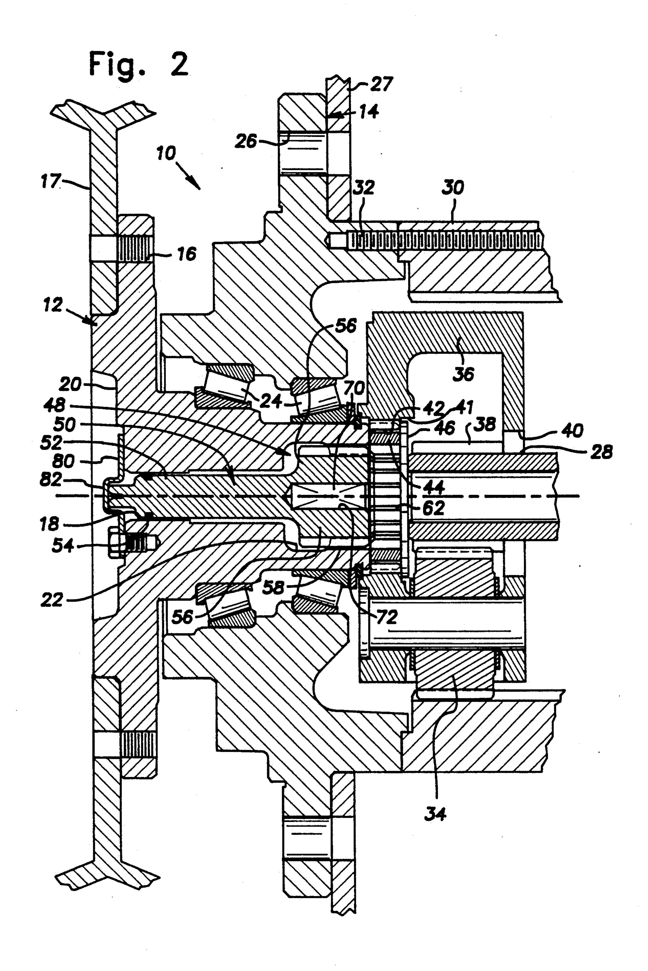
be towed at normal highway speeds since rotation of the spindle does not cause rotation of the gear train.
