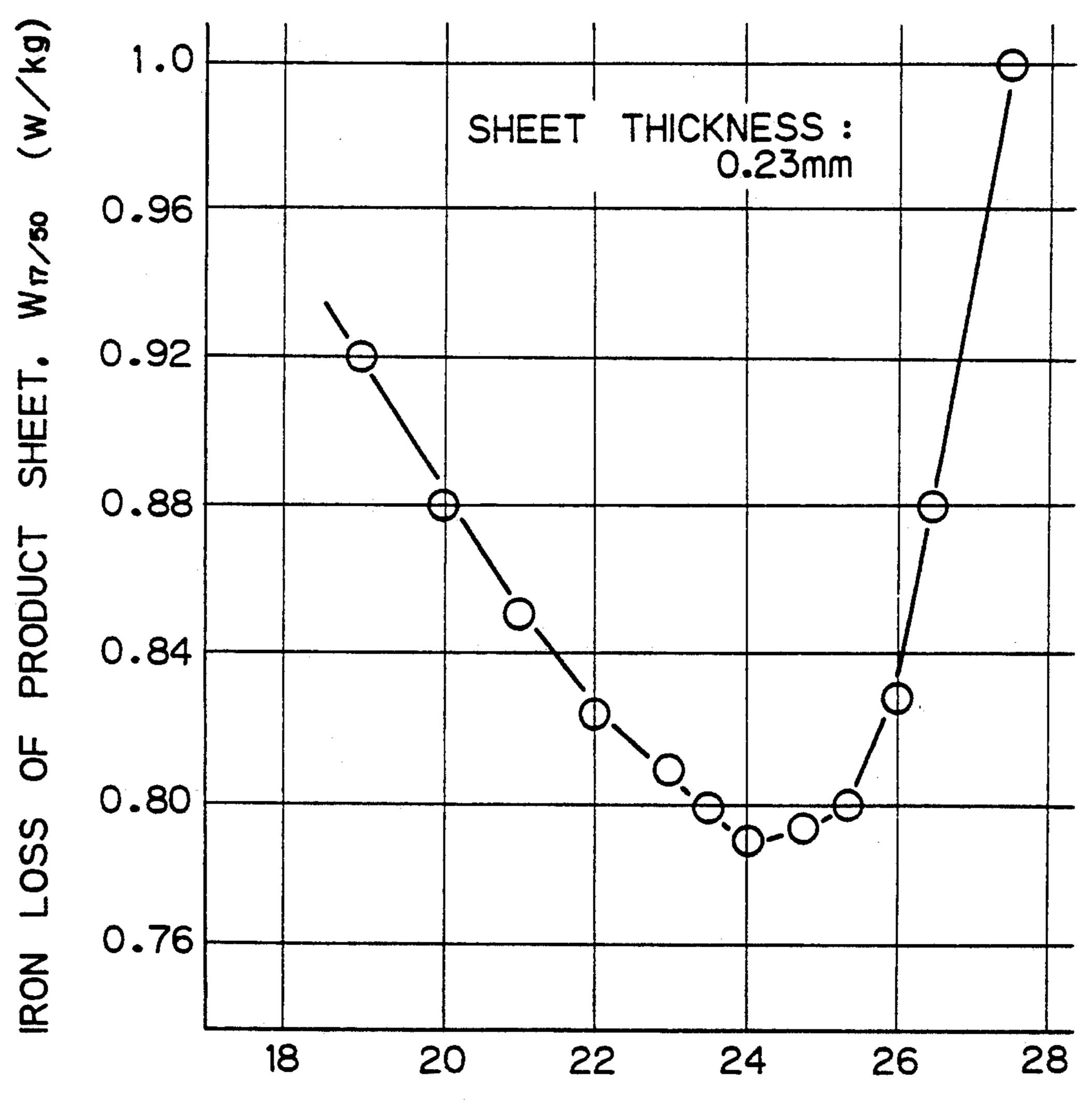
AVERAGE DIAMETER OF PRIMARY RECRYSTALLIZED GRAIN AFTER DECARBURIZATION ANNEALING (µm)
