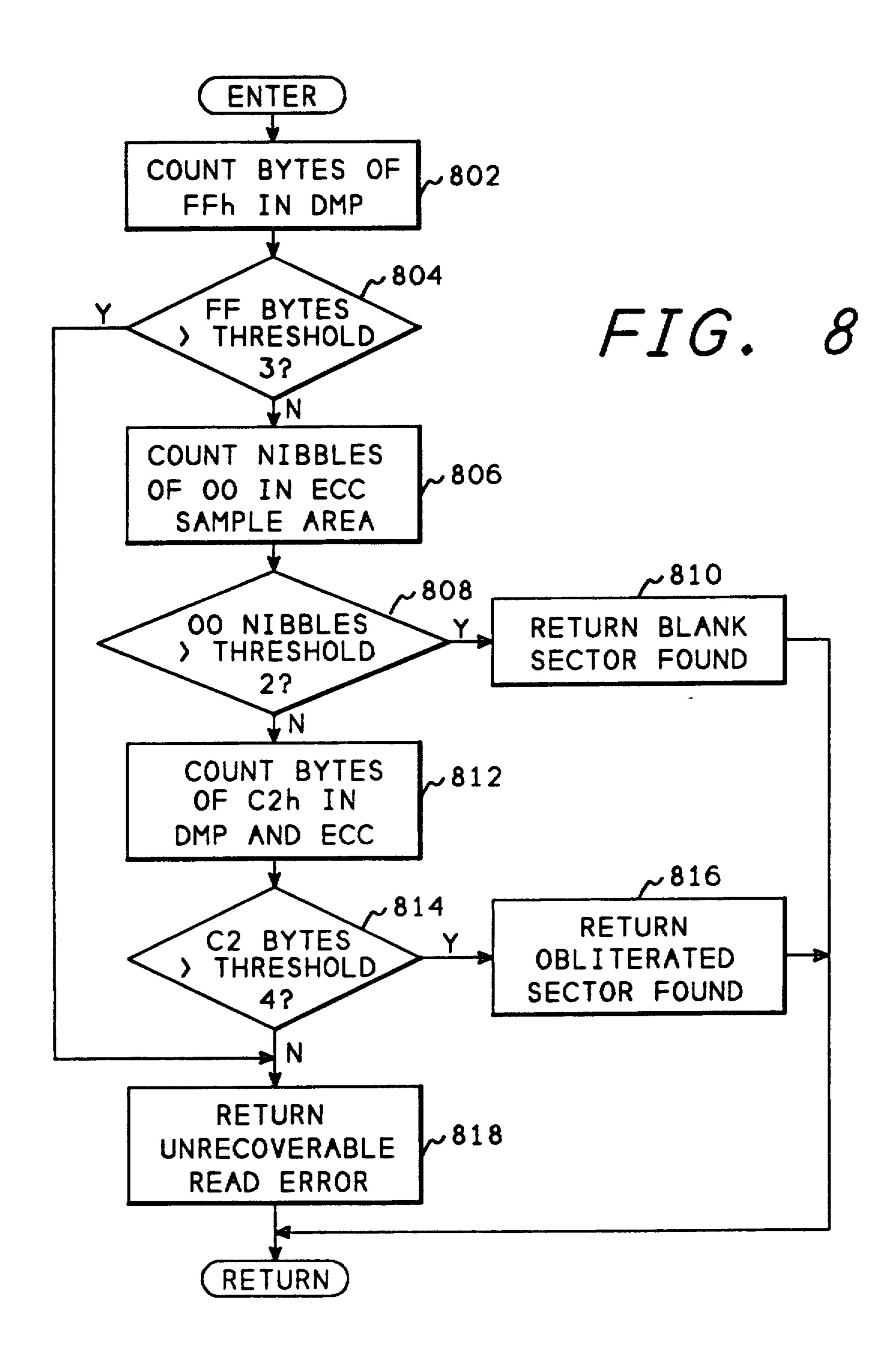
METHOD AND APPARATUS FOR DETERMINING SECTOR STATUS IN A DATA STORAGE DEVICE BY WRITING A STATUS OF READ-ONLY, WRITABLE, OR OBLITERATED IN AN ERROR RECOVERY AREA OF EACH SECTOR
