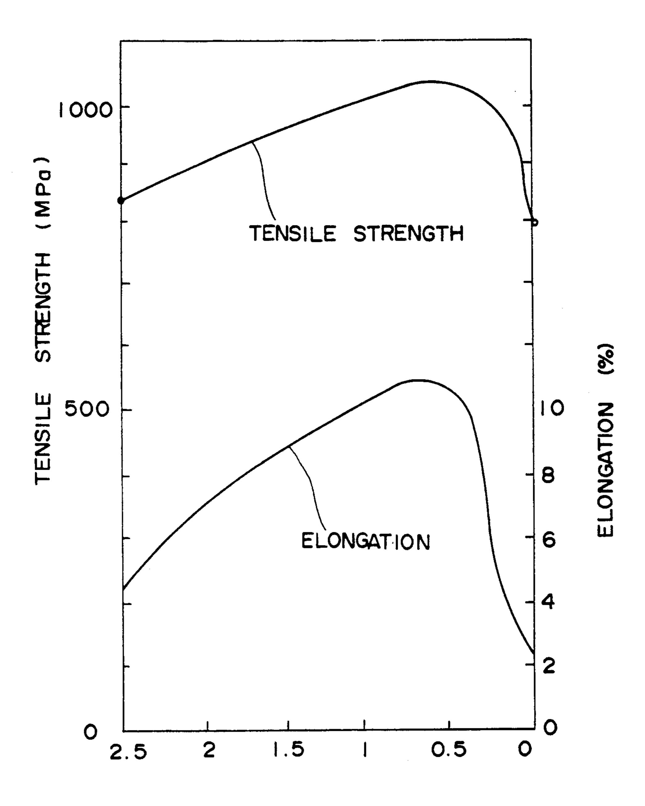
Zr content (x), at.% (Algo.5Ni7Mm $_{2.5-x}$ Zr<sub>x</sub>)
